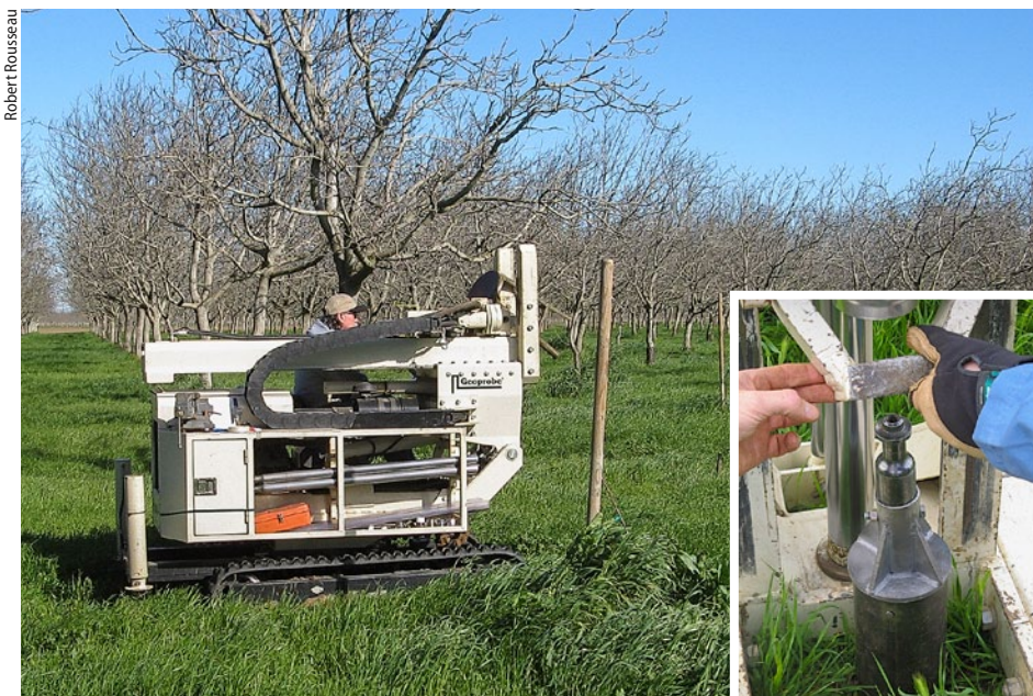
Geoprobe sampling at Dixon Ridge Farms organic walnut orchard. Inset, geoprobe soil core sampling to a depth of 39.4 inches (1 meter).
