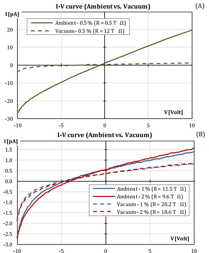
Fig. 7. (A) Voltage vs. current curves for the electrospun PCL with 0.5 wt% of graphene, (B) voltage vs. current curves for the electrospun PCL with 1 wt% and 2 wt% of graphene.
