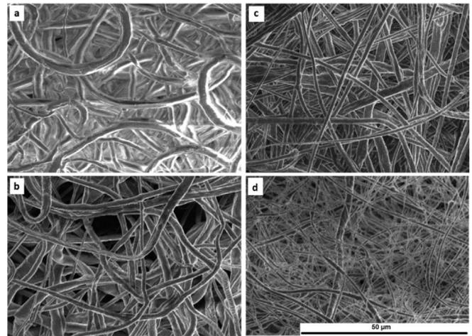
**Fig. 2.** SEM images (1200 $\times$ ). (a) THF:DMF with 0 wt% graphene, (b) THF:DMF with 0.5 wt% graphene, (c) THF:DMF with 1 wt% graphene (d) THF:DMF with 2 wt% graphene.
