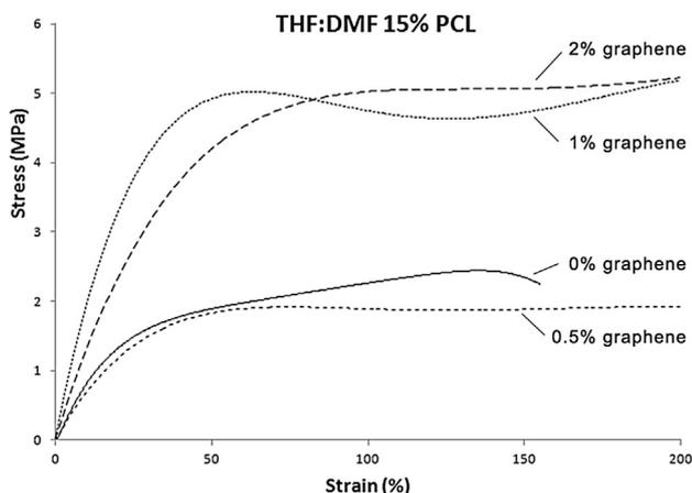
Fig. 6. Tensile engineering stress vs. engineering strain curves for the electrospun PCL with different contents of graphene nanosheets.
