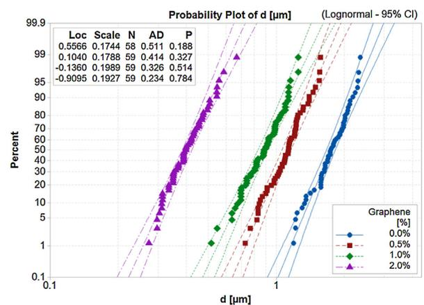
**Fig. 4.** Probability plots of the fiber diameter distributions using a lognormal distribution.
