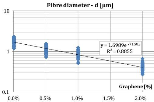
Fig. 5. Influence of the graphene content on the fiber diameter, interpolating line and correlation coefficient ( $R^2$ ).
