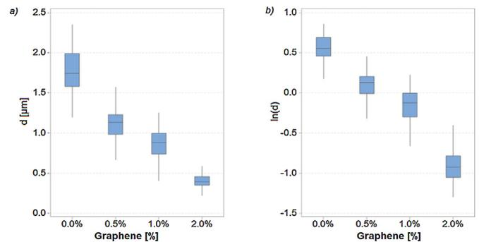
**Fig. 3.** Influence of the graphene content on the fiber diameter. Box plots of (a) direct measures and (b) logarithmic measures.
