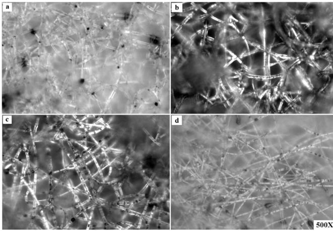
**Fig. 1.** Optical microscope images (500 $\times$ ). Comparison between preliminary dispersion tests: (a) 0.5 wt% of graphene is added to THF:DMF–PCL solution, (b) PCL is added to the THF:DMF–graphene solution with 0.5 wt% of graphene, (c) 1 wt% of graphene and (d) 2 wt% of graphene.
