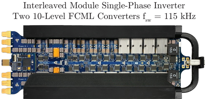
Fig. 3. A top-down view of an InterLeaved Module (ILM). Each PCB contains two, interleaved 10-level FCML converters switching at a frequency of 115 kHz with LC filters on board. ILM electrical characteristics are given in Table II
