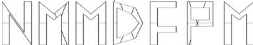
Fig. 3. Generated mesh by tree cutting with coarser and denser triangular meshes with the two alternative methods to represent fractures.
