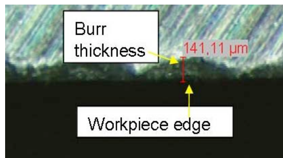
FIGURE 3. MEASUREMENT OF BURR HEIGHT AND THICKNESS.
