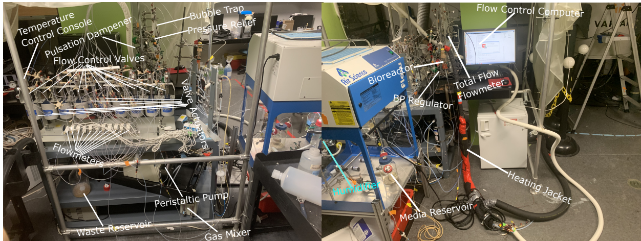
Figure 2.5: Bioreactor System Setup. Full view of the system setup. Each photo comprises a half of the system.
