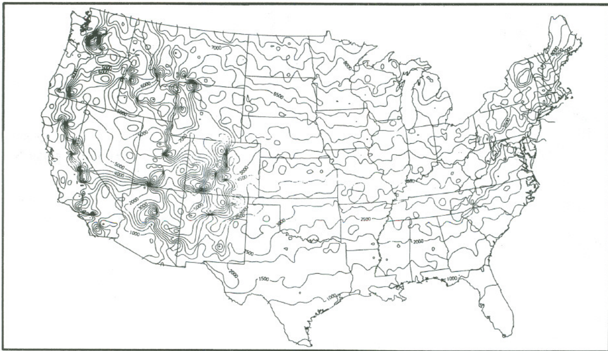
Fig. 5.2.4 Heating Degree Days at 60F Base Temperature 30-year average (1950-1980) for 3200 NOAA stations XBL 856-2934
