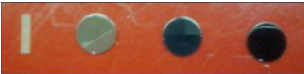
Figure 3.3. TiO 2 samples of increasing reduction, the color change is attributed to the accumulation of Ti 3+ defects. The approximate number of cleaning cycles conducted on each sample from left to right is 0, 3, 12, 50 cycles.
