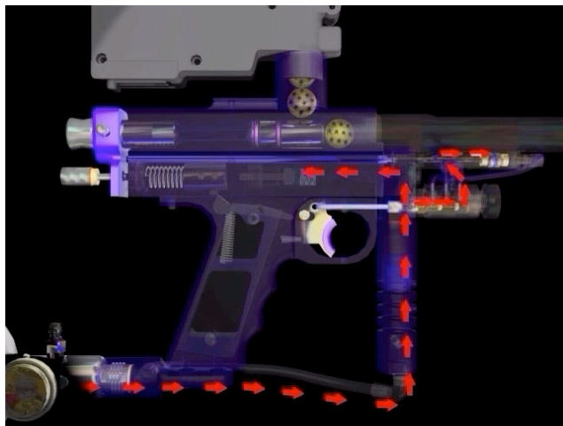
Figure 8. Air Flow in Paintball Gun
