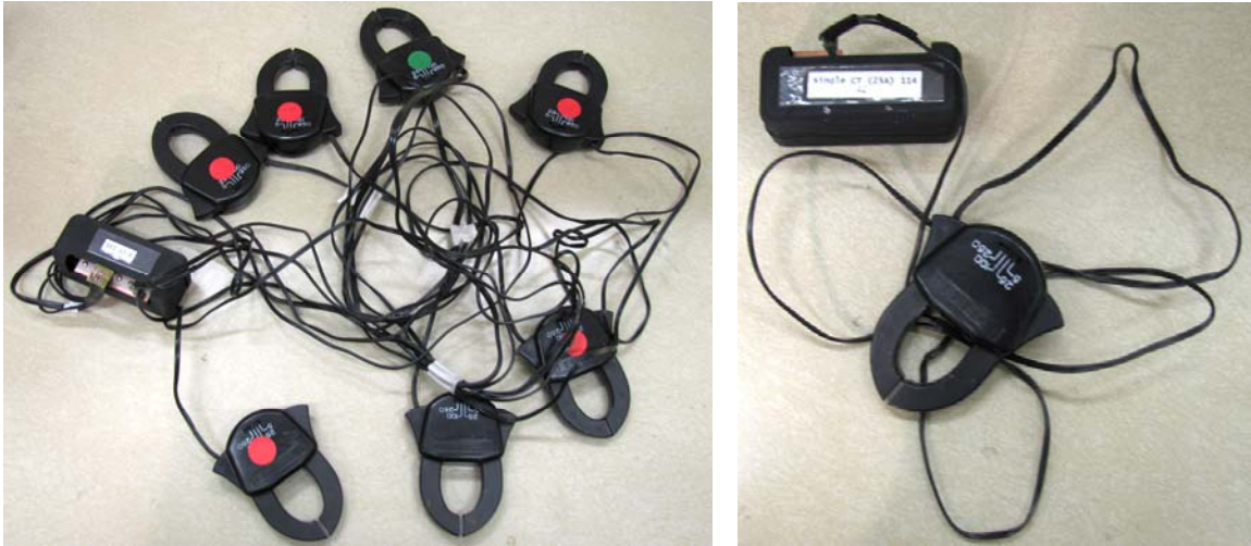
Figure 33: Current sensors for the circuit breaker panel (left) and for an individual appliance cord (right). 52
