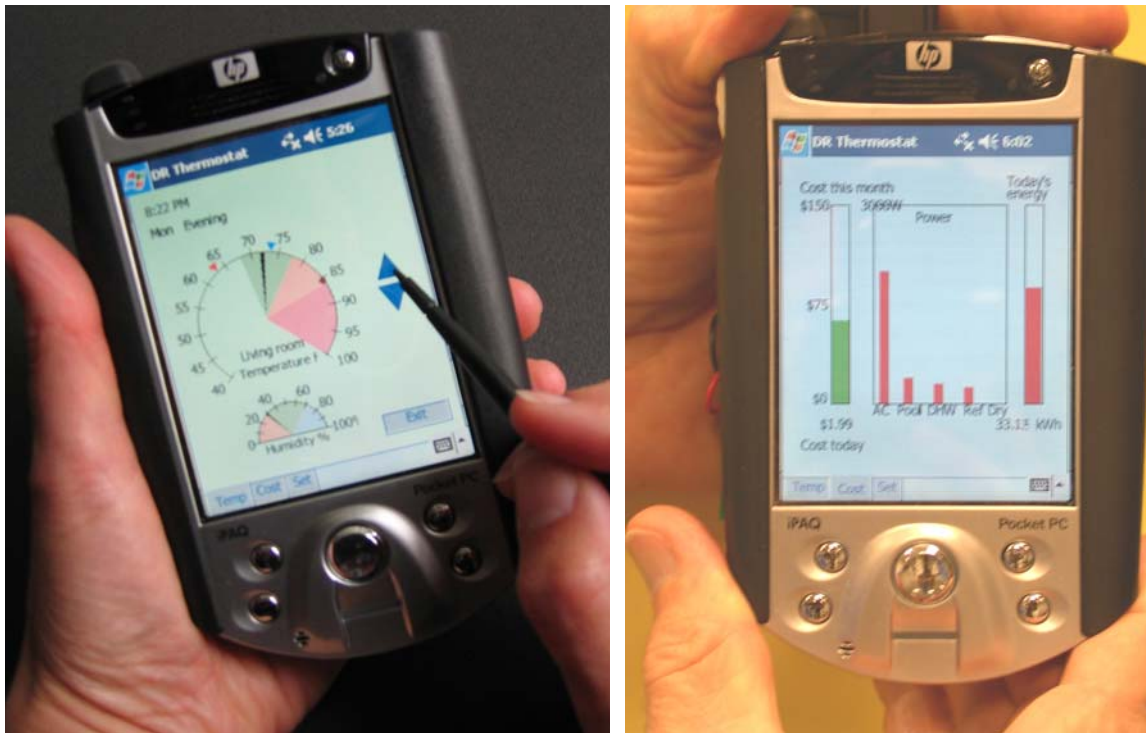
Figure 57: The early DREAM user interface showing temperature (left) and energy, cost, and power information (right).
