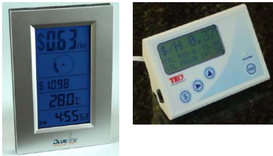
Figure 21: Left: Blue Line Monitor, Right: The Energy Detective.
