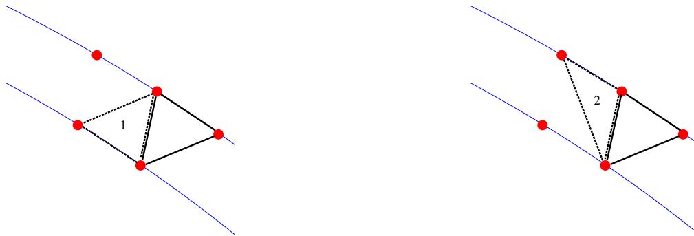
Figure B.1: The original triangle pick in between two flux surfaces is plotted with solid lines, and the next two potential triangles are plotted with dotted lines.
