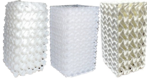
Figure 5: Resin, PC, and PLA specimens at different print densities of the gyroid infill pattern.
