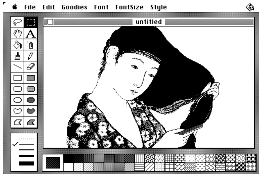
Figure 5.6: Bill Atkinson's MacPaint (1984). Released with the Apple Macintosh. Note tool palette at left. Illustration by Susan Kare, based on a Japanese woodcut (Kare 2001). Source: Wikipedia. The overall interface design builds upon GUI conventions cultivated at Xerox PARC. These GUI conventions—developed with children as a primary audience—were invented and refined in order to produce software that was both easy to use and facilitated creative activity (Hiltzik 1999; Waldrop 2001).
