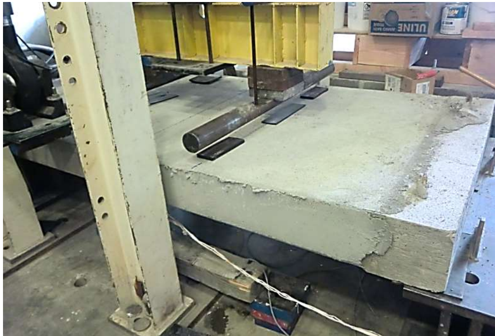
Figure (4.8): Side View of Slab Set-up prior to Testing [11]
