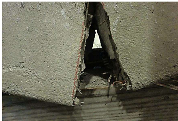
Figure (4.10): Up-Close Failure of Cold Rolled Wires In The Center Of CSP without additional Hot-rolled reinforcement [11]
