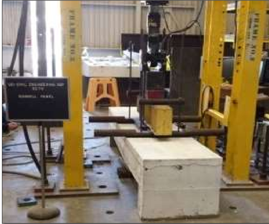
Figure (4.3): Side View of Slab Set-up prior to Testing [11]
