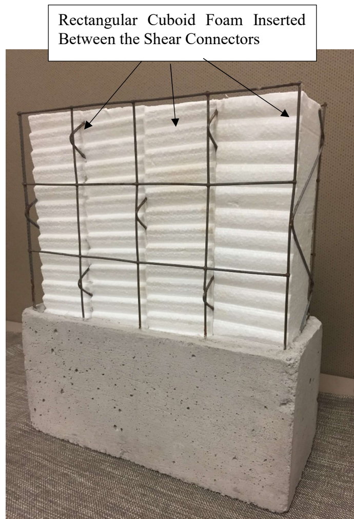
Figure (2.4): One of the First Designs of CSP With Continues Truss Shear Connectors
