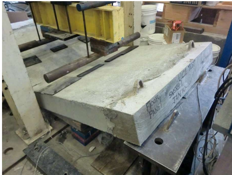
Figure (4.9): Brittle Failure Of CSP Specimen Without Additional Hot-Rolled Reinforcements [11].
