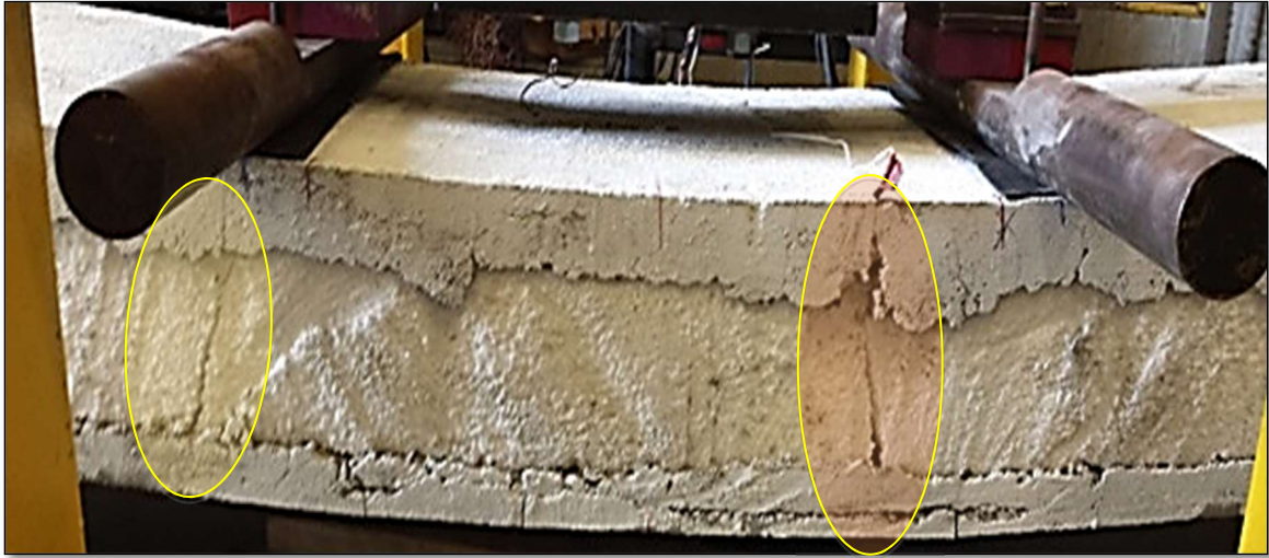
Figure (4.4): Cracks due to Flexure at Mid-Span for Specimen Parallel-CSP
