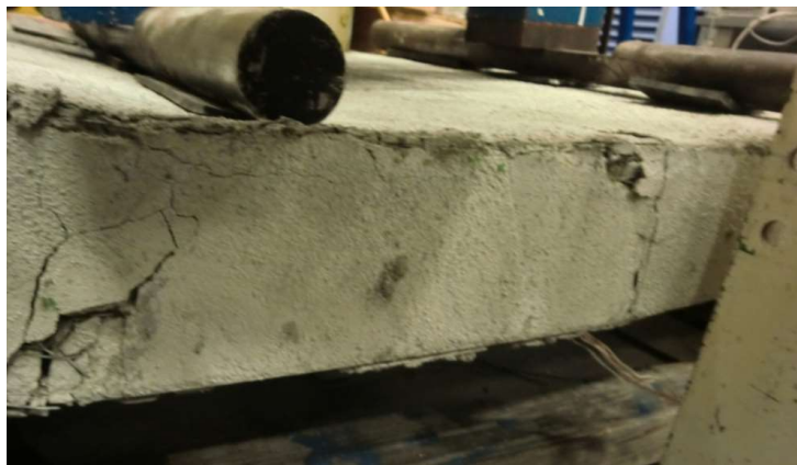
Figure (4.11): Shear Failure of Diagonal CSP Specimen at 45° Degree Angle and Flexural Cracks at Centerline of Specimen at Ultimate Load. [11]
