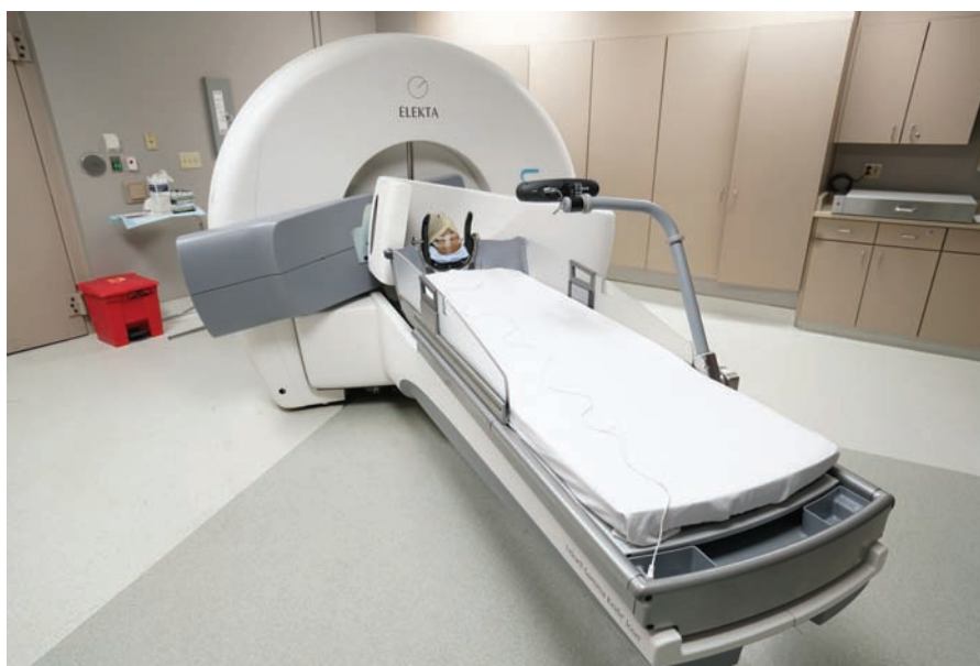
Fig. 1 Gamma Knife Icon system with a retractable 90 kV CBCT unit mapped in submillimeter stereotactic coordinates for treatment setups. Shown is the starting position of the CBCT arm for online imaging acquisitions. This picture is provided by Dr Dheendra Prasad, Rosswell Park, Department of Radiation Oncology.
