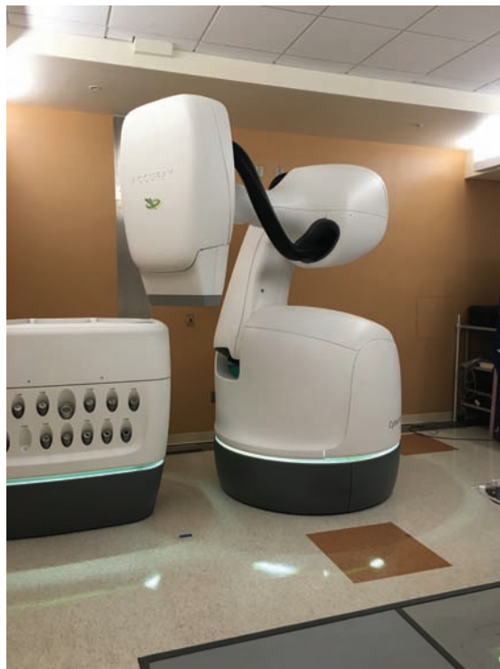
Fig. 2 The Cyberknife M6 which is equipped with the InCise2 high definition MLC (leaf width = 3.85 mm at 80 cm SAD) allowing for a maximum clinical field size of 11.5 × 10 cm 2 . Picture provided by Dr Lei Wang of Stanford University, Department of Radiation Oncology.
