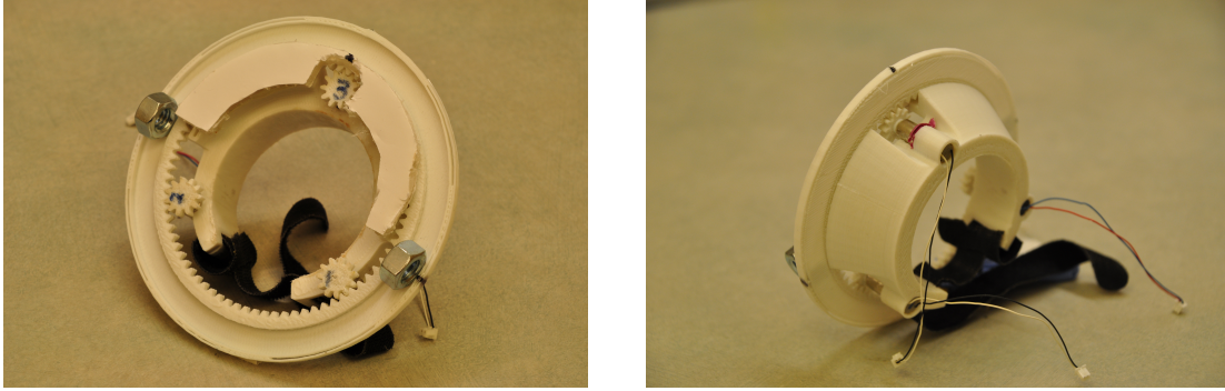
Figure 4.12: Front and back of the tremor suppression device. This 3D-printed device features a weighted reaction wheel that is used to dampen Parkinsonian tremor. The strap at the bottom of the device allows for easy mounting to the mechanical test rig developed in Section 4.2.
