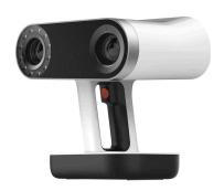
This portable system projects patterns, whose deformation is read realtime and aligned with SLAM to create 3D scans.
