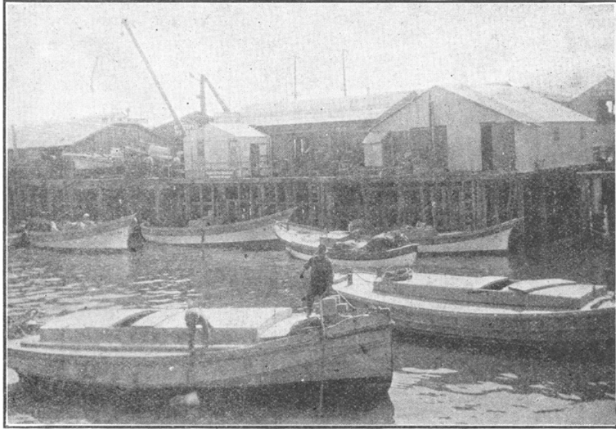
FIG. 10. Round-bottomed lighters in foreground, sardine launches in background. Photograph by W. L. Scofield, Monterey, 1919.
