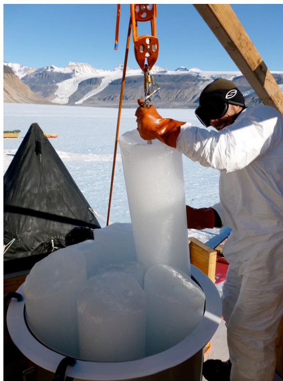
FIG. 13. Large-volume ice sampling for ^{81}\text{Kr} dating at Taylor Glacier. The ice cores are 24 cm in diameter and the mass of ice being loaded into the vacuum extraction vessel is ~ 300 kg. Photo credit: V.V. Petrenko.
