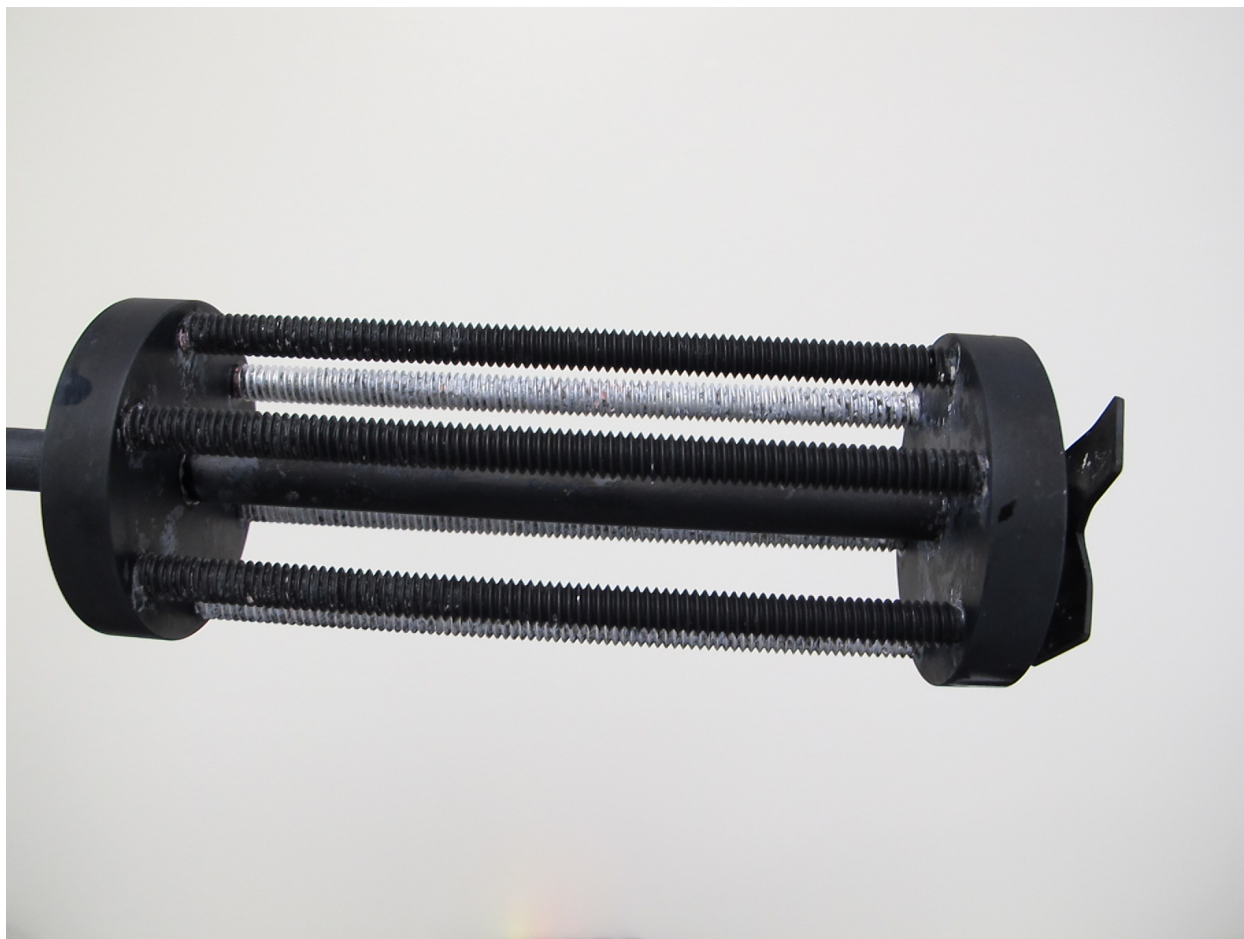
Figure 3.6: Custom spindle for fibers to wrap around. The spindle is built to ensure proper mixing of the catalyzing solution while reducing surface contact with the fibers.
