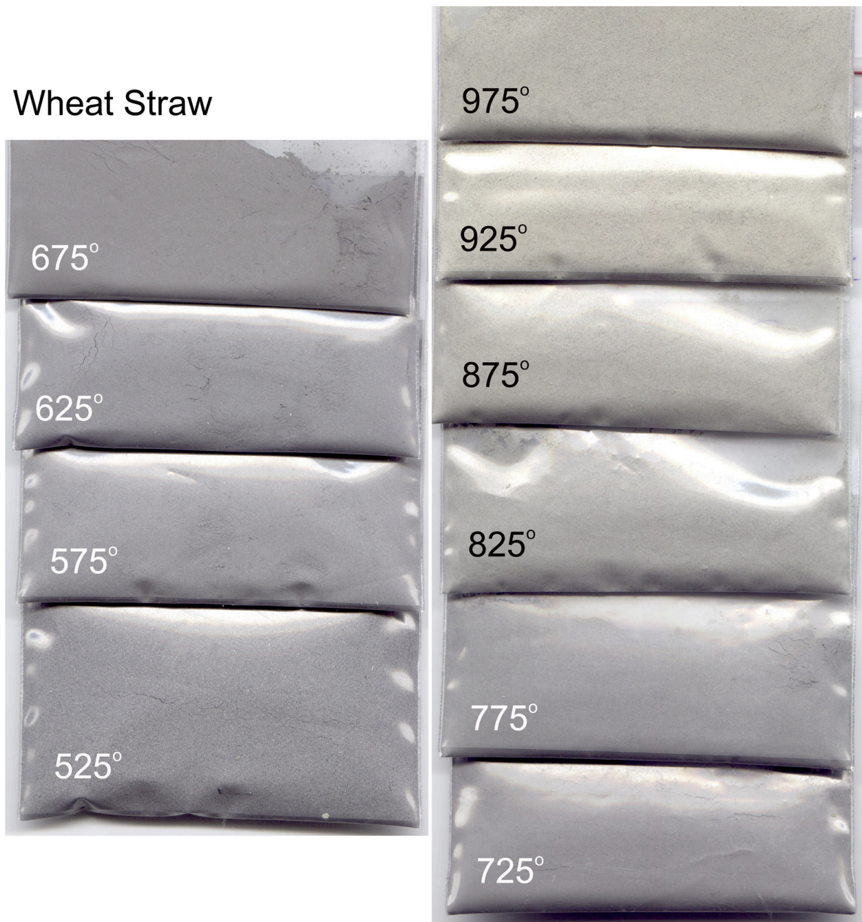
Figure 4. Color variation of powdered experimental ashes and slag from wheat straw. Experimental temperature is given in degrees Celsius and is the uncorrected set point values. The powdered ashes and slag are contained in plastic bags. Color variation is given in Table 2.
