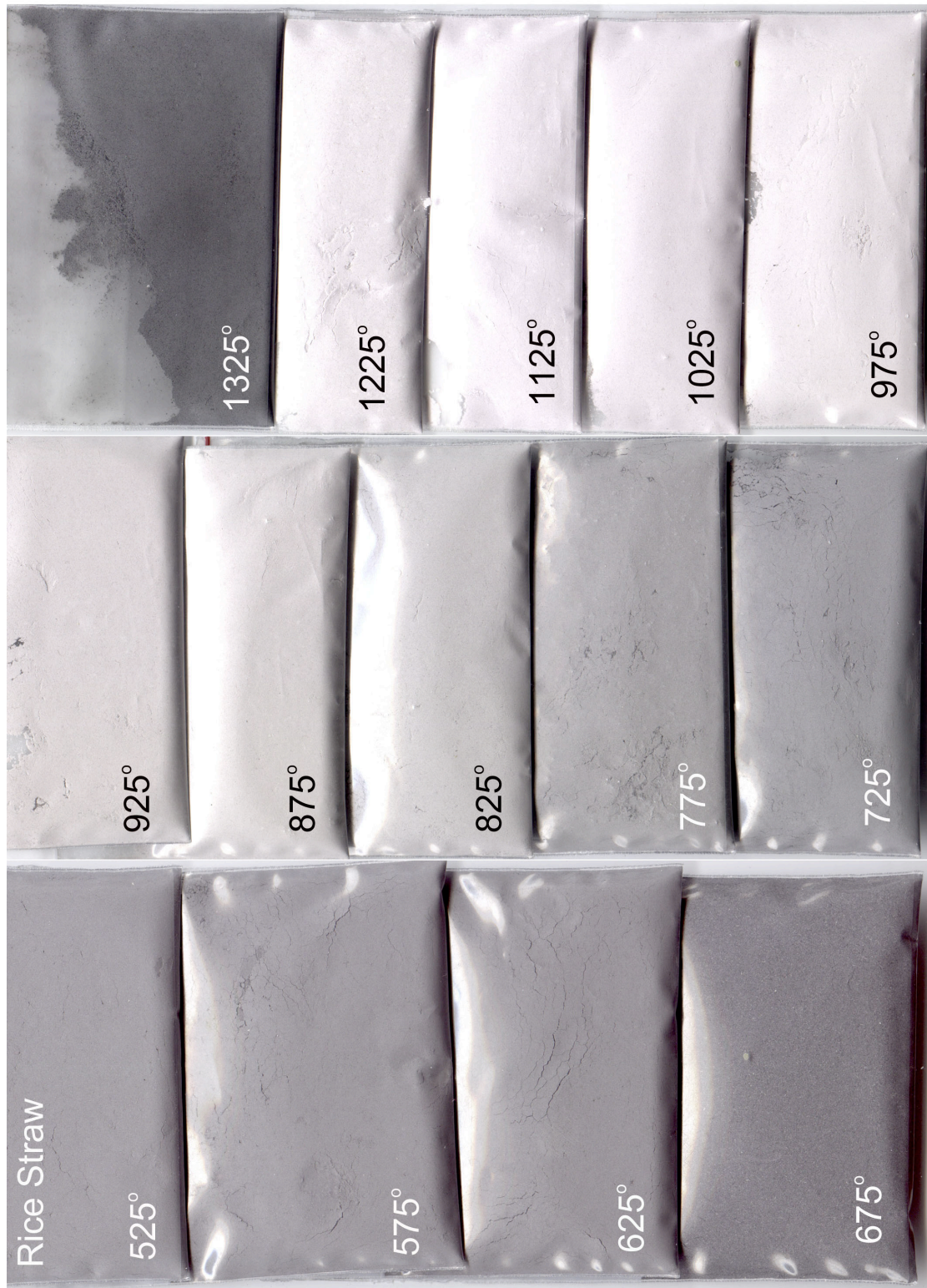
Figure 3. Color variation of powdered experimental ashes and slag of rice straw. Experimental temperature is given in degrees Celsius and is the uncorrected set point values. The powdered ashes and slag are contained in plastic bags. Color variation is given in Table 2.
