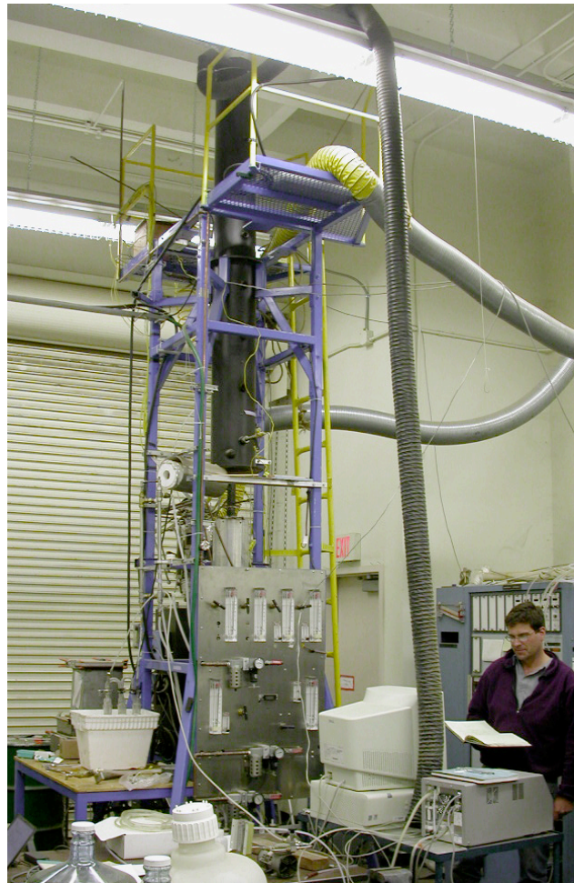
Figure 6A. The laboratory scale fluidized bed combustor at University of California, Davis. This combustor was used by Thy et al. (2004) for controlled experiments that provided fly ash samples for the present study.
