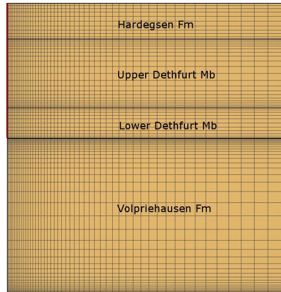
Figure 1. 2D window of the radial model with four geological layers (Petrasim interface). The injection well is located at the left side and does not penetrate the VP Fm.
