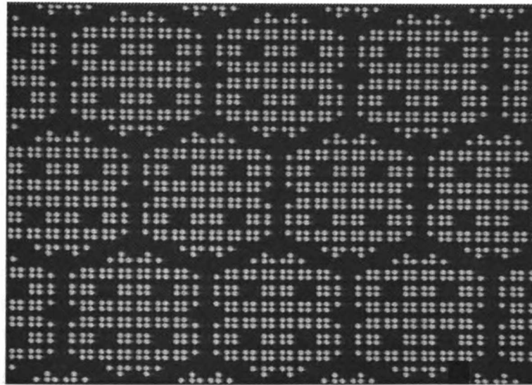
Figure 9.2.3 A micrograph of the Design II cell culture wafer. The etched holes on the filter membrane are 3 \mu\text{m} in diameter and the actual 78 nm diffusion channels are underneath.
