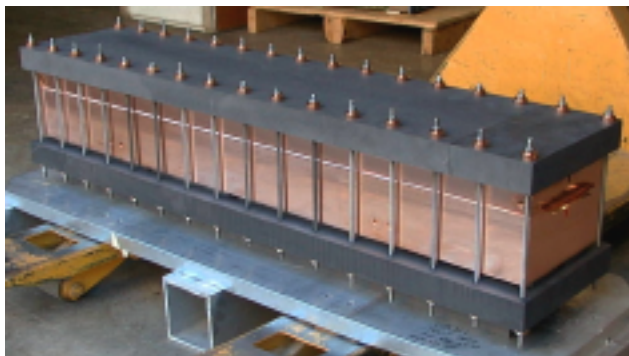
Figure 2 – RFQ clamping arrangement for GlidCop® to copper braze.
