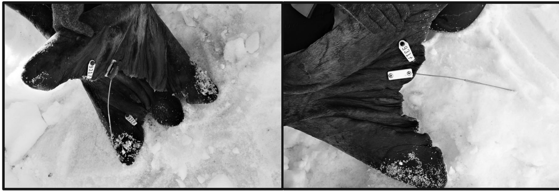
Figure 2. Dorsal (left) and ventral (right) views of prototype flipper tag with very high frequency transmitter after 341 days of attachment to Weddell seal flipper in McMurdo Sound, Antarctica, during the Austral Summer 2015. Upon tag removal, flipper holes were well-healed with no evidence of pressure necrosis or irritation, demonstrating an improvement over conventional flipper-tag attachments.
