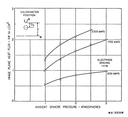
Fig. 7. The thermal flux at the image plane as measured with the continuous flow calorimeter.
