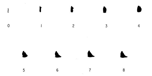
Fig. 9. High speed photographs of arc plasma development.
