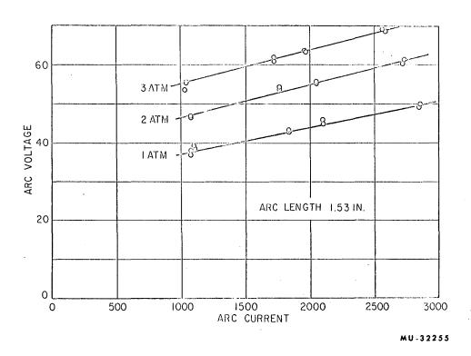
Fig. 4. Electrical characteristics of the argon arc.
