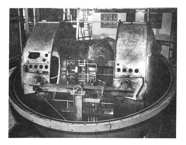
Fig. 2. Interior view of the environmental sphere showing the mirror mounting and arc electrodes. The receiver assembly is not visible, but is located at the focal point of the mirror on the right.
