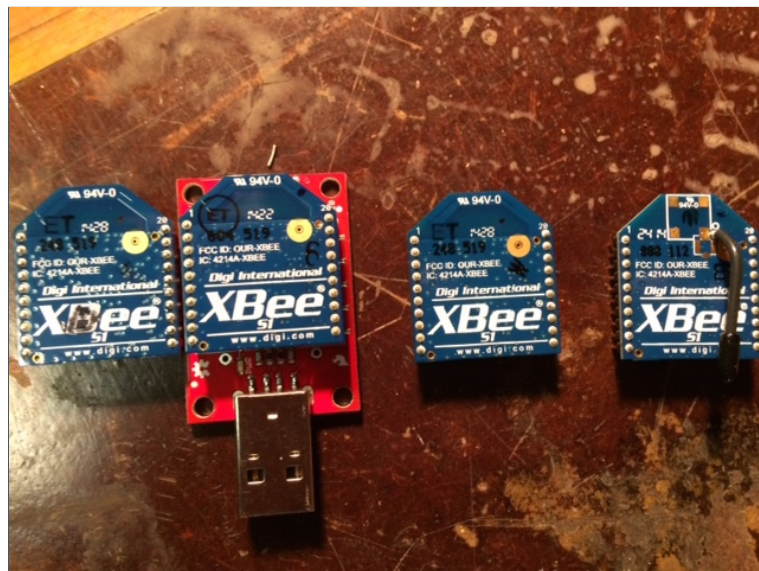
Figure 4.17: Picture of Xbee units deployed on MIST platform, with Xbee Explorer (for programming the units) in red. See Fig. 4.18 for location of units on model.
