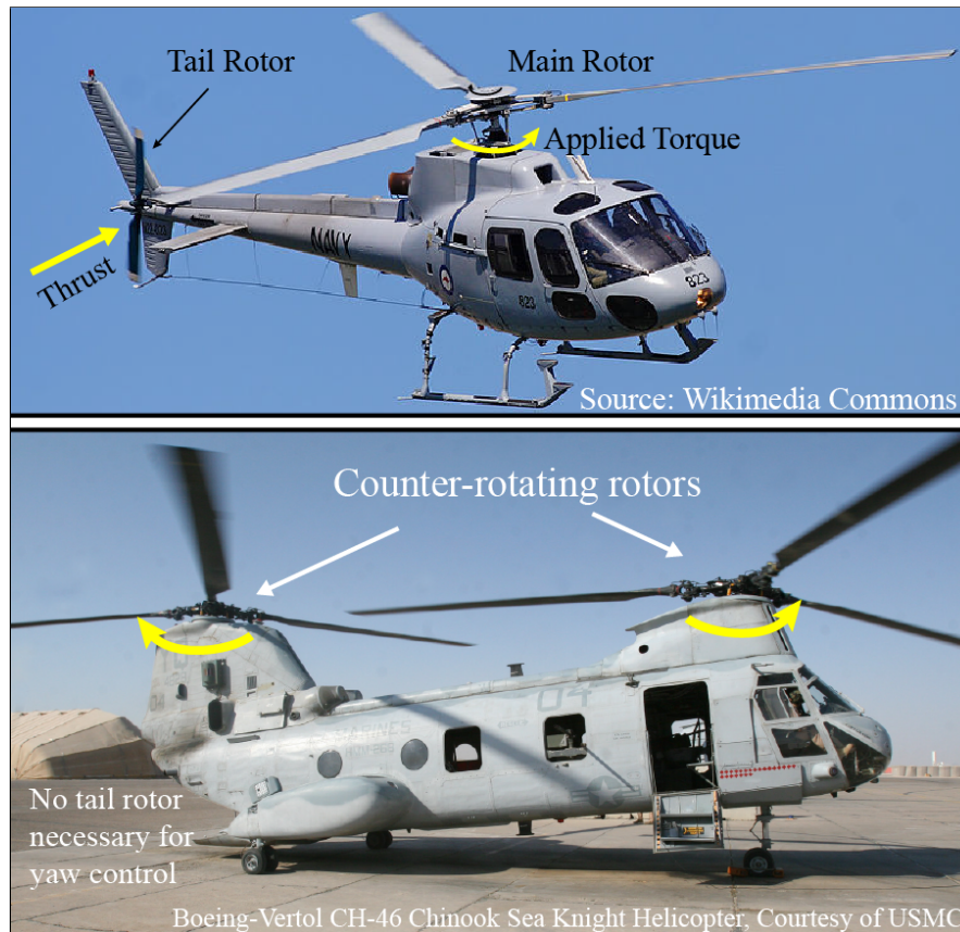
Figure 6.1: Single rotor with tail rotor and tandem rotor helicopters with counter-rotating rotors.
