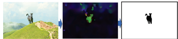
Figure 1: Illustration of our system to detect and localize digital manipulations. The manipulated image on the left is processed through a bank of resampling detectors to create a heatmap (middle), which is then used by a classifier to detect/localize the modified regions (right)
