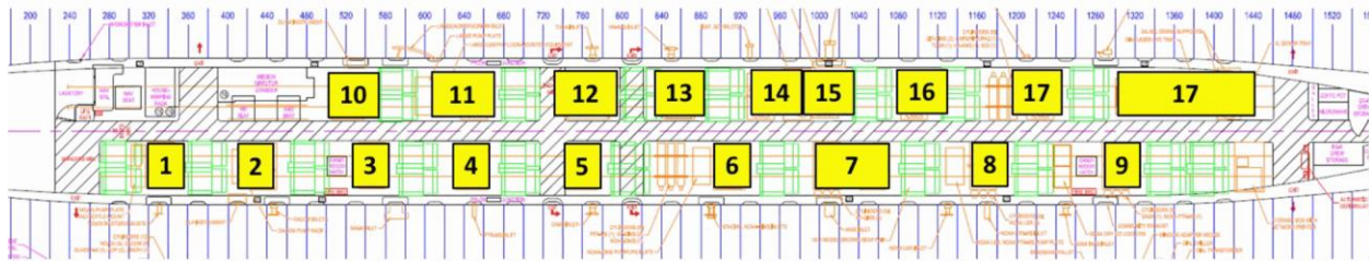
Figure 2.2 Seat and instrument layout for the DC-8 cabin during FIREX-AQ (Adapted from FIREX-AQ White Paper, 2018).
