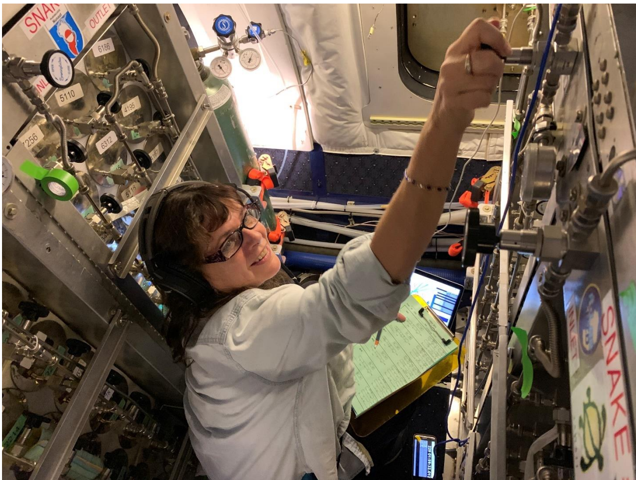
Figure 2.6 Dr. Nicola Blake collecting a whole air sample during the FIREX-AQ campaign. In this photo Dr. Blake has her hand on the outlet valve.
