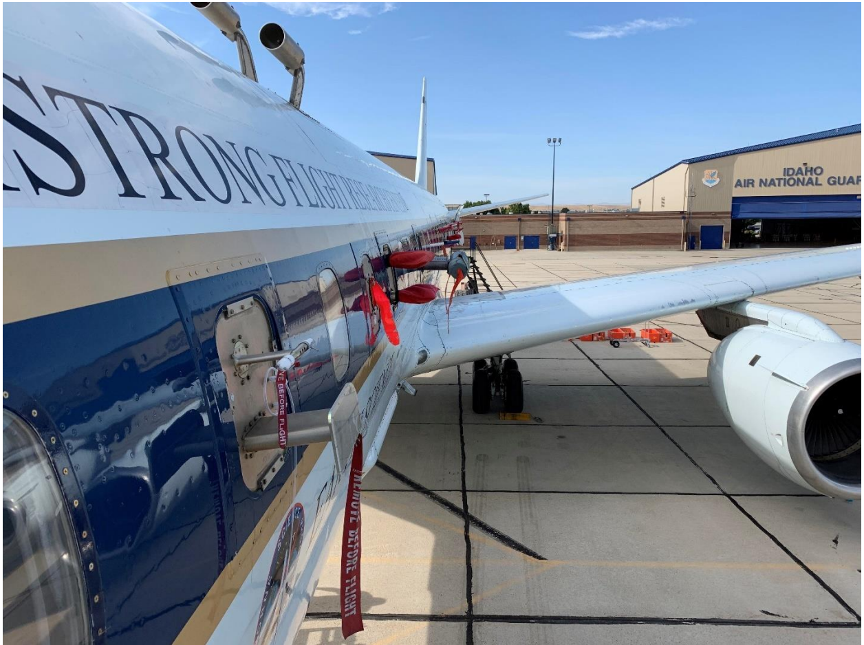
Figure 2.5 Picture of the outside of the fuselage of the DC-8, showing the inlets and ports mounted to the aircraft. The port side and underside also have inlets and ports for instruments (not pictured).
