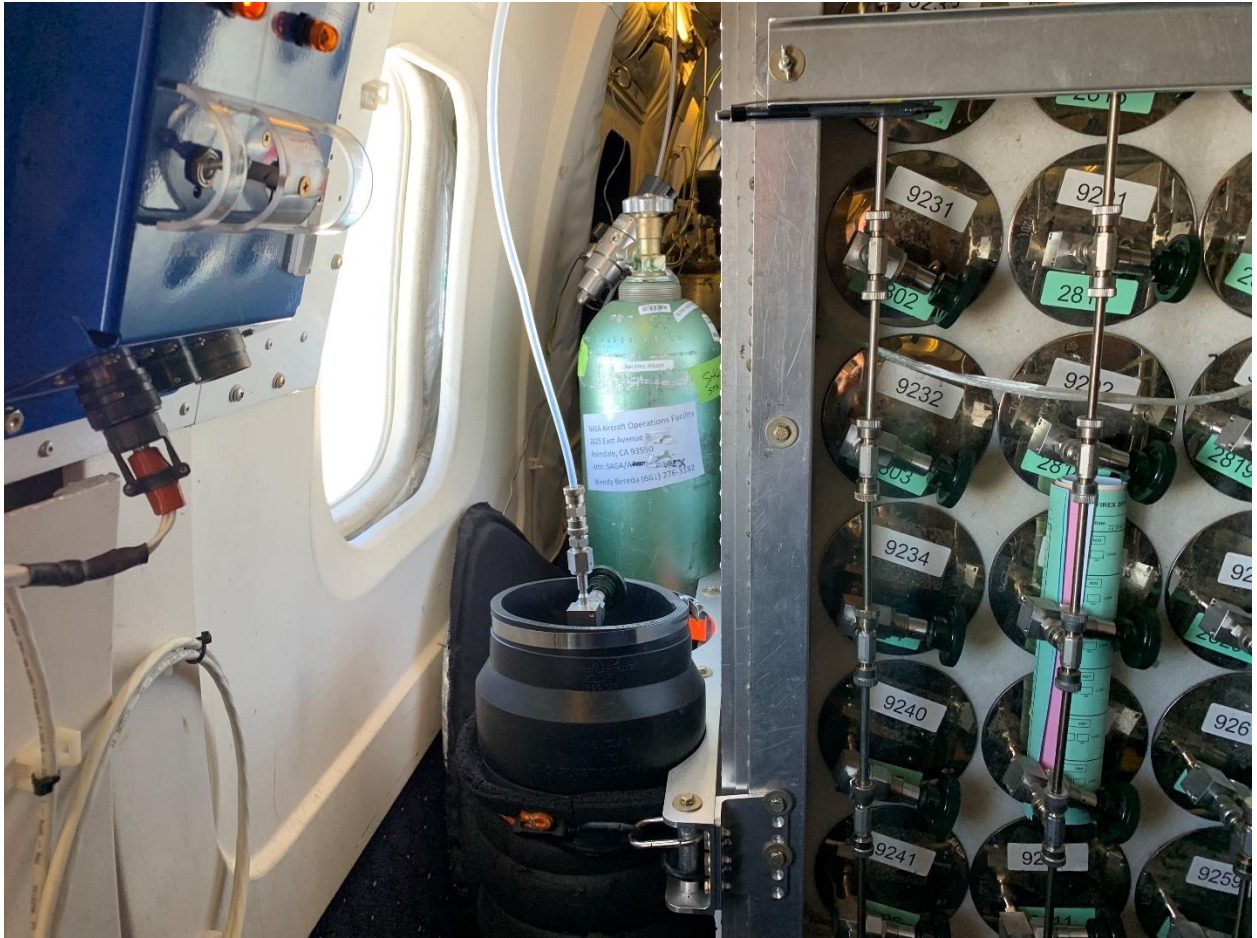
Figure 2.7 Photo taken during the 2019 FIREX-AQ campaign showing the location of the pontoon used for pressure testing on the fuselage side of the rearmost rack. To the right is a new snake loaded into the caddy, with the data collection sheets rolled and set in the snake for use.
