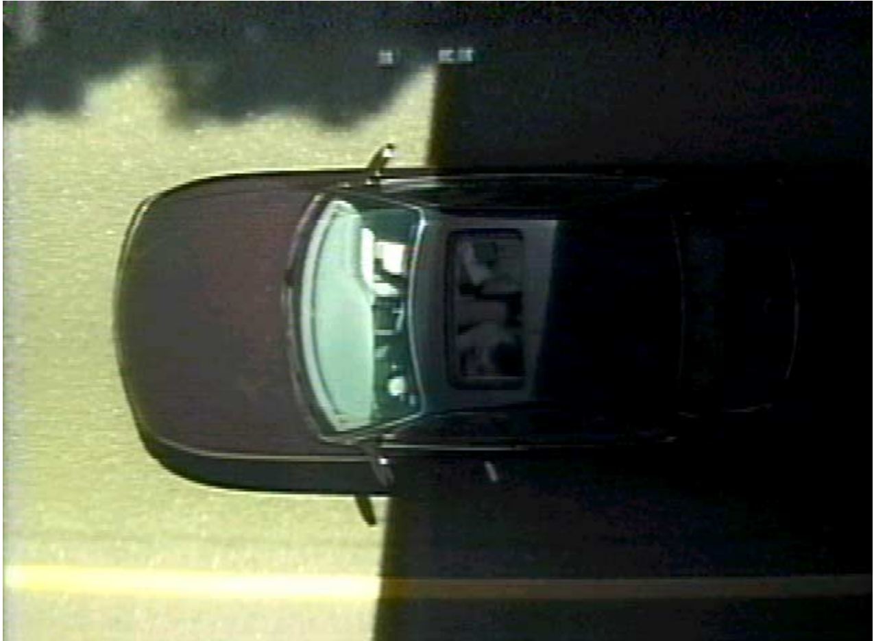
Figure 25. Camera sensitivity set low. Result is loss of intensity information in shadowed area.
