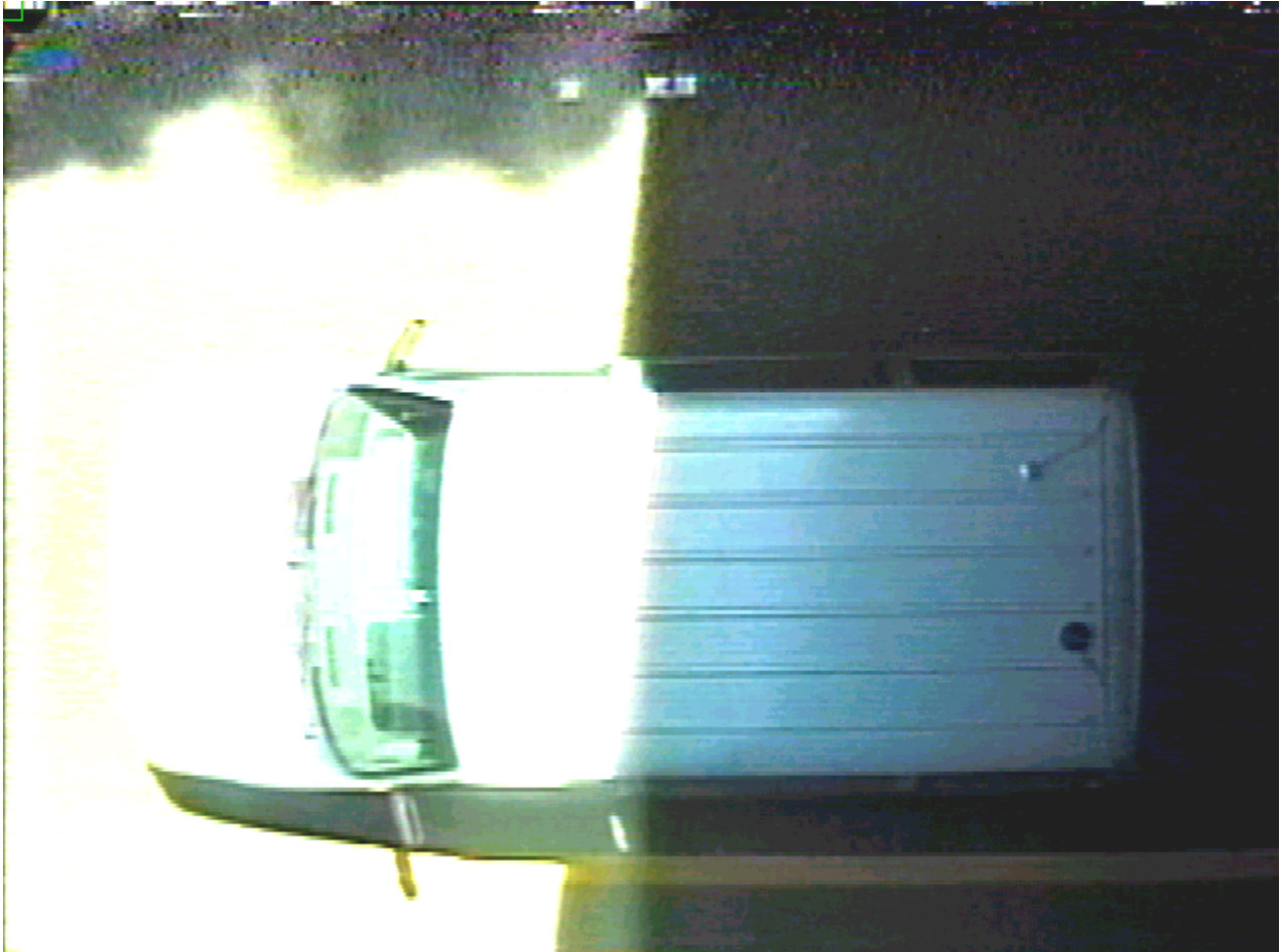
Figure 24. Camera sensitivity set high. Result is saturation of sunlit areas.
