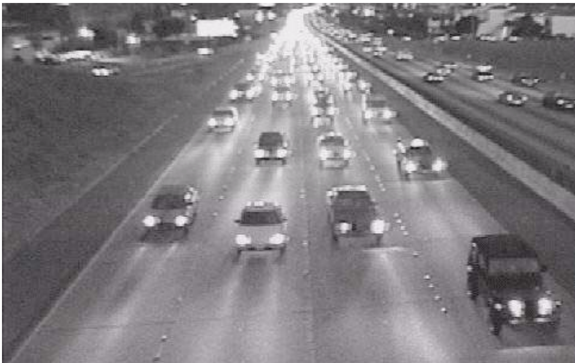
Figure 15. Digitized Video Image of Night Highway Traffic, Burle TC9388-1 Camera, Auto-shutter mode.
