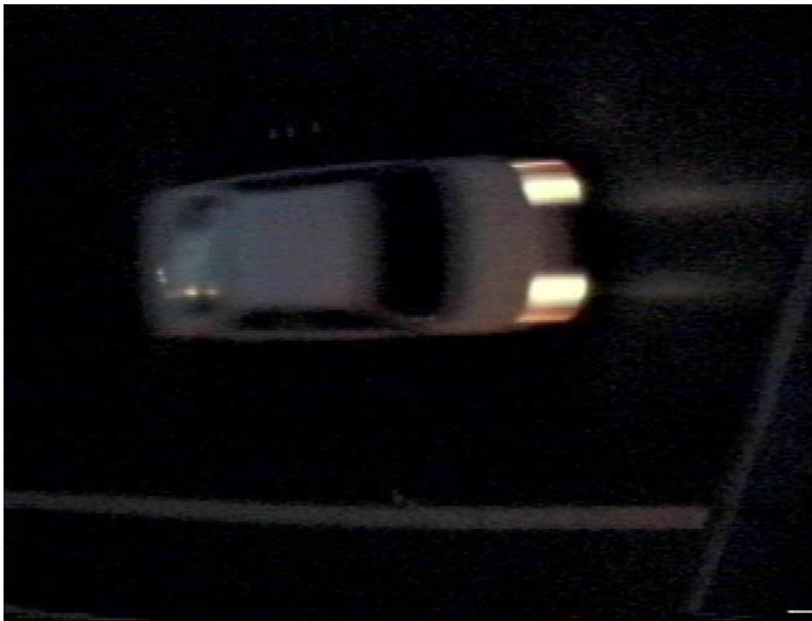
Figure 10. Image Blur Due to Slow Shutter Speed Under Low-Light Conditions.
