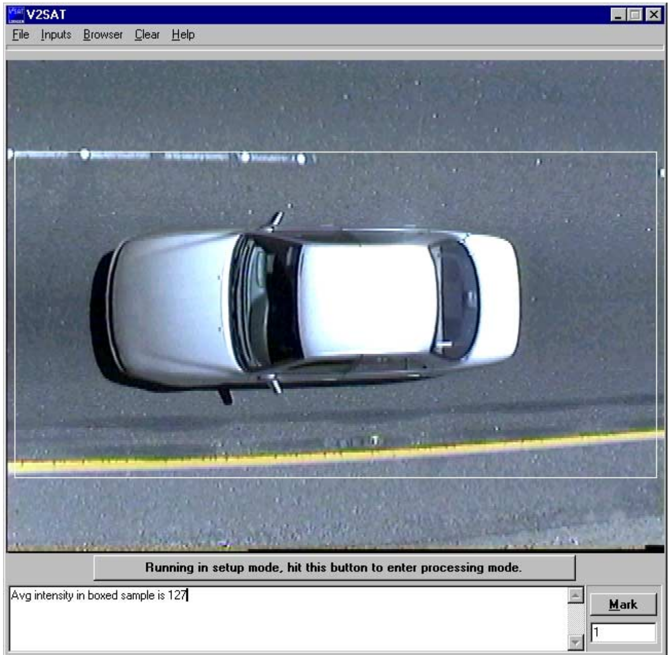
Figure 16. Example of Proper Camera View and Detection Window Placement.
