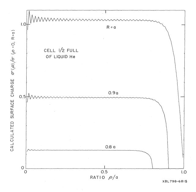
Fig. 4. Plot of the calculated surface charge density for several values of the charge pool radius. The plots are normalized to the surface charge density at the center of the cell when the entire surface is covered with charge. The oscillatory structure at the center of the charge pool is an artifact of the finite element approximation.
