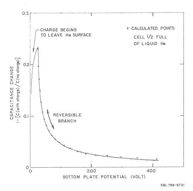
Fig. 6. Comparison between the measured curve of capacitance change versus voltage and the results of our electrostatic calculation. The discontinuity of slope in the measured curve occurs when the charge pool begins to flow off the surface onto the walls.
