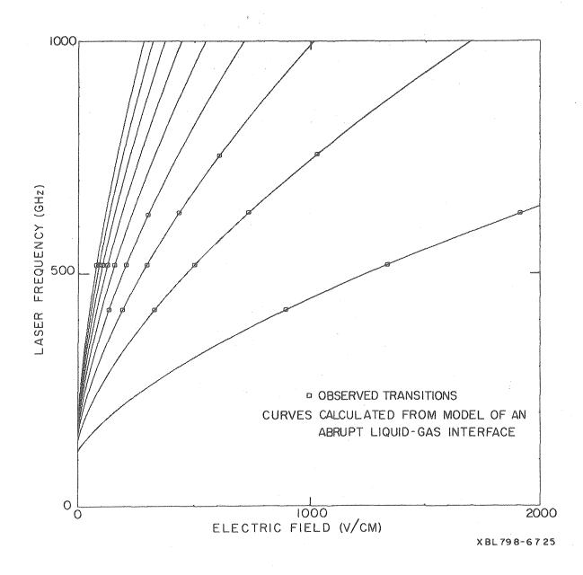
Fig. 12. Plot of the laser frequency versus electric field at which transitions are observed. The curves are the same as in Fig. 1.
