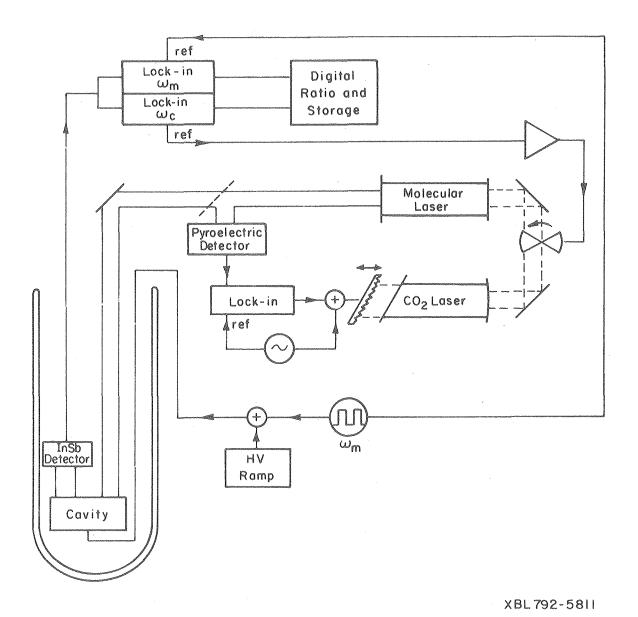
Fig. 7. Block diagram of the apparatus used for optical measurements.
