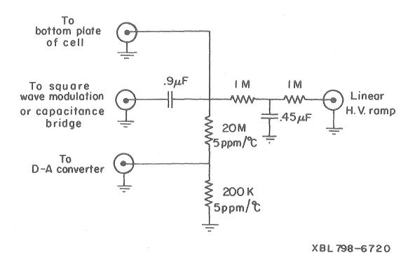
Fig. 9. Circuit used to apply modulation voltage to the bottom plate of the cell.
