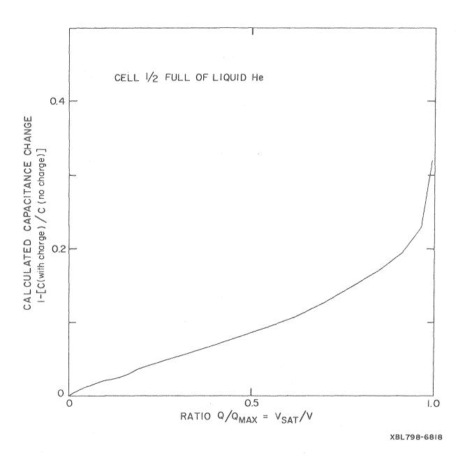
Fig. 5. Calculated capacitance change versus total charge on the helium surface. The maximum amount of charge,  $Q_{max}$ , corresponds to covering the entire surface with the charge pool.
