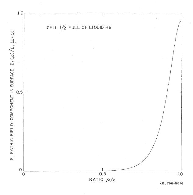
Fig. 3. Plot of the external electric field in the plane of helium surface (which confines charge in the charge pool) as a function of radial distance. The plot is normalized to the electric field along the axis of the cell.
