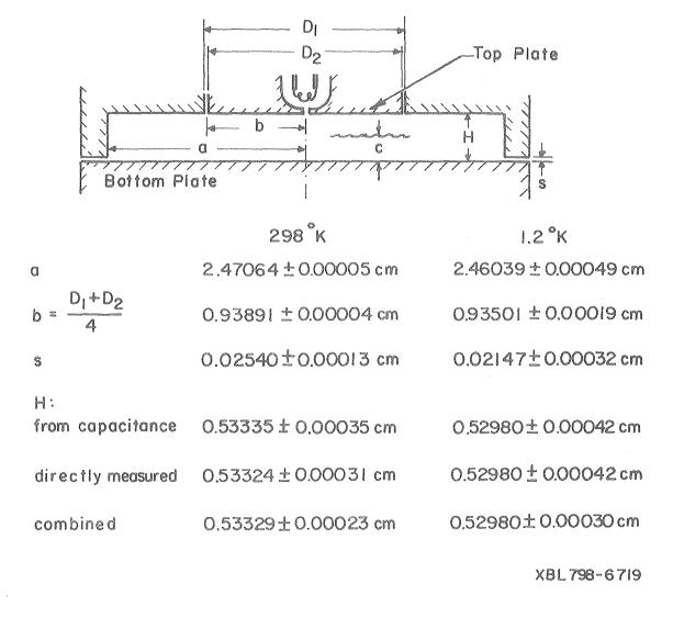
Fig. 2. Cross-section drawing of the cylindrical cell within which electrons are confined on the helium surface.
