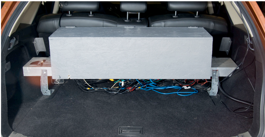
Figure 4.2: Computer enclosure in luggage compartment behind rear seat of vehicle, with cover closed.
