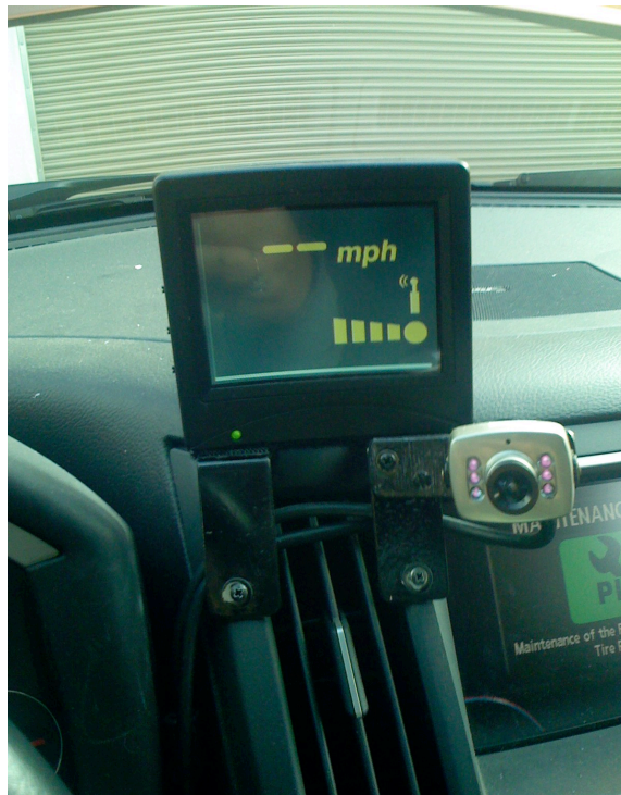
Figure 3.25: CACC display (right of steering wheel)
