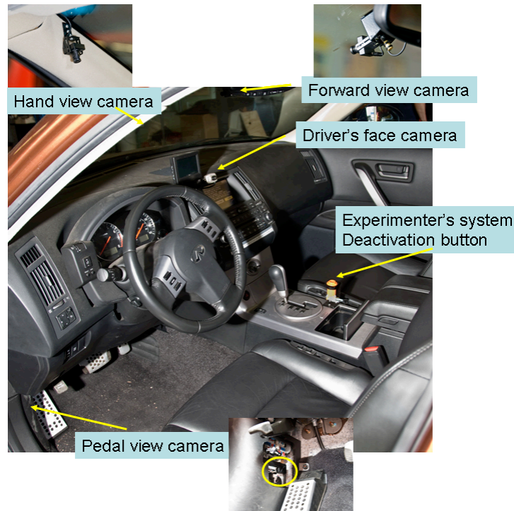
Figure 4.4: Vehicle Interior, Showing Locations of Video Cameras
