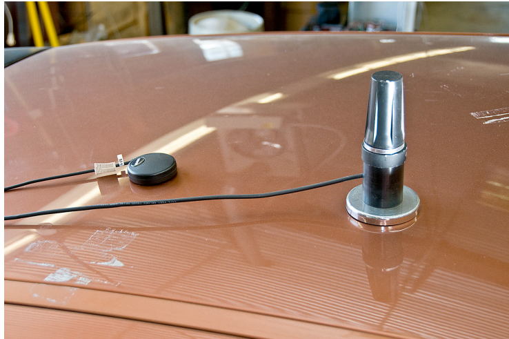
Figure 4.3: DGPS Antenna (left) and DSRC Communication Antenna (right)
