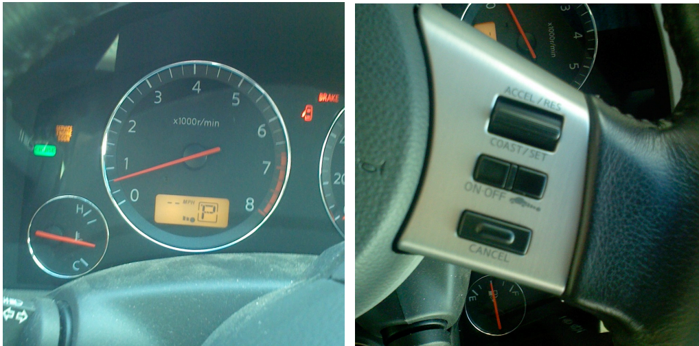
Figure 3.24: ACC displays (left) and controls (right)
