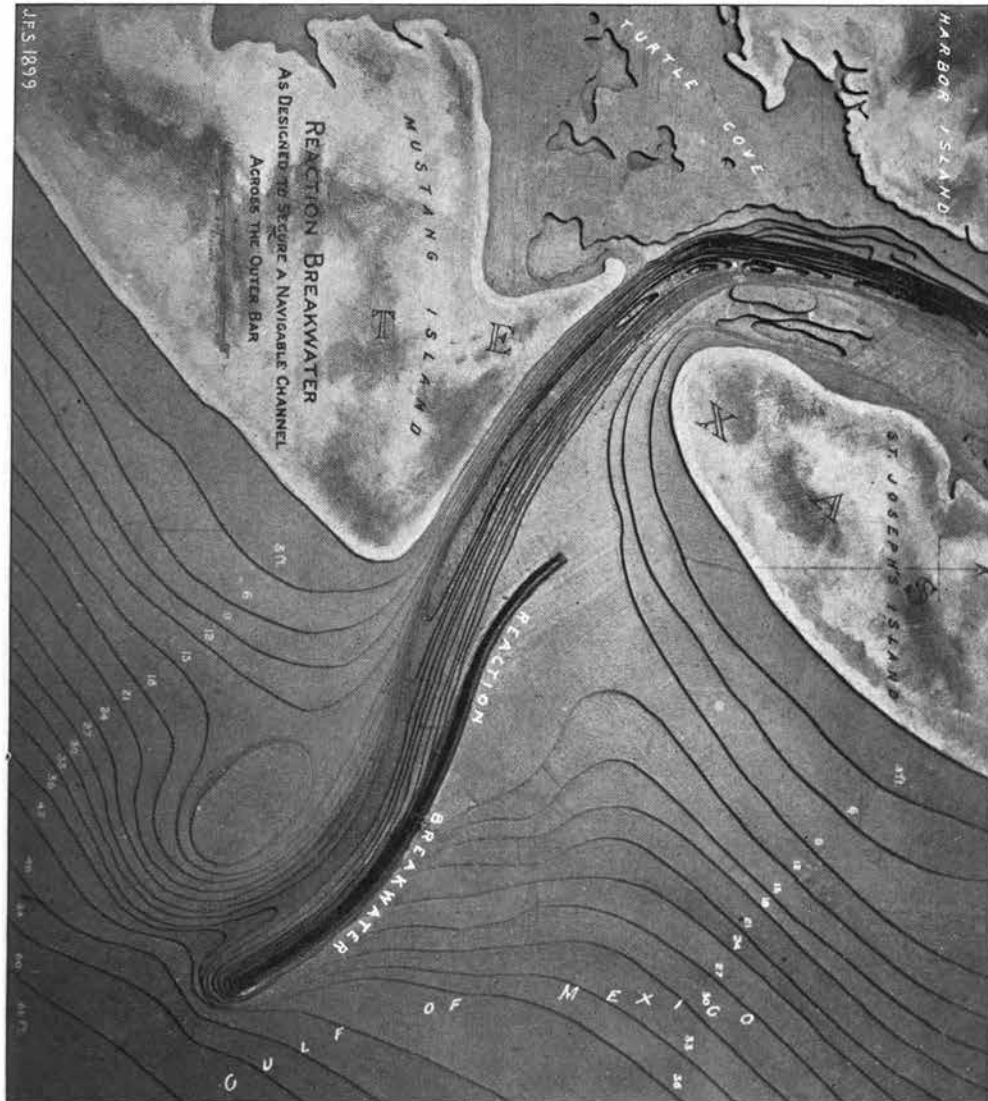
PROBABLE CONDITION OF BAR TO BE EFFECTED BY THE COMPLETION OF THE REACTION BREAKWATER AND REMOVAL OF OBSTRUCTING JETTY.
