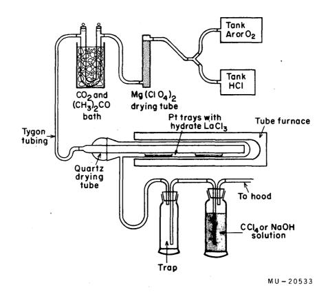
Fig. 12. Apparatus used to dry rare earth trichlorides. Tank HCl and Ar were passed through a drying tube to remove water, and through a carbon dioxide-acetone bath to remove certain organic material in the tank HCl.
