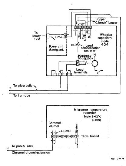
Fig. 16. Wiring diagram of Wheelco controller and temperature-recording unit.
