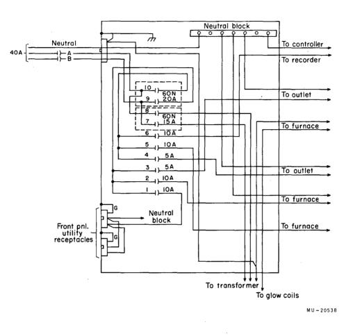
Fig. 15. Wiring diagram of power rack.
