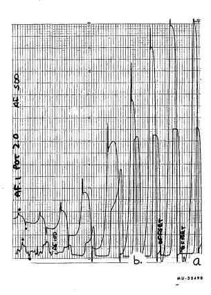
Fig. 80. Curves similar to those in Fig. 79 illustrating the consistent behavior of the WHG and the strange behavior of the thermocouple probe, which actually remains at a constant level between (a) and (b) while the WHG signal decreases by 35%. The fact that the signals from both measurement devices decline as the air is flushed from the bubbler and rotameter again demonstrates that water is ineffective in this system. P = 81 mtorr and t = 20 sec/small div (right to left). (March 6, 1965).
