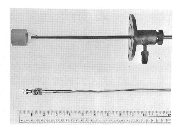
Fig. 14. Photograph of movable probes used with Wilson-seal and ratchet assembly: (a) a long water-cooled glass-tube and Teflon-sleeve assembly to hold metal or glass disks (top), and (b) a long glass tube for internally heating a metal resistance wire.
