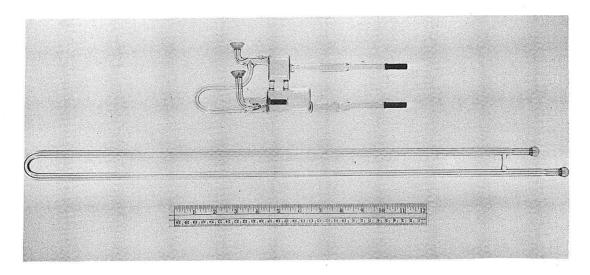
Fig. 4. Photograph of the complete mercury-plug flowmeter showing the relative sizes of the mercury-housing part and the 3-mm i.d. capillary tube.
