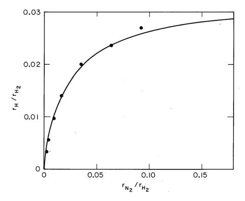
Fig. 66. The effect of high  $N_2$  flow rates on the yield of atoms from a low-pressure (80 mtorr  $H_2$ ) 50-MHz discharge (20% dial setting). The pronounced saturation and the low yield of atoms per  $N_2$  molecule show that  $N_2$  is much less effective than  $O_2$ . The concentrations of H and  $N_2$  are plotted relative to the amount of  $H_2$  in the entering gas stream. (January 31, 1965).
