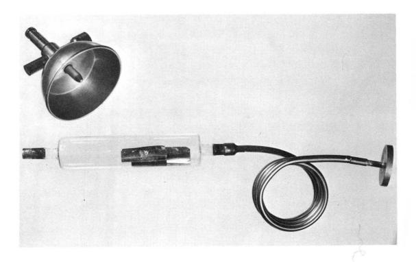
Fig. 12. Photograph of (a) the Burdick Type A reflector, which was used with (b) the oxygen-to-water converter consisting of a 40-mm o.d. 15-cm long glass tube and 8-mm o.d. 45-foot long copper tubing internally electroplated with nickel.
