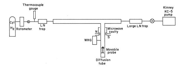
Fig. 21. Schematic drawing of preliminary apparatus. The rotameter leaked.
