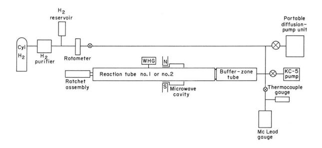
Fig. 24. Schematic drawing of diffusion-tube apparatus. The rotameter leaked, so that the "purified" hydrogen was in fact contaminated with an unknown amount of air.
