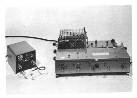
Fig. 22. Photograph of the complete Decker-Lamers-Rony differential micromanometer showing the modified Decker pressure transducer (on left) and the Laboratory-designed electronics. This unit had a short-term stability of 1  $\mu$ torr and a long-term stability of 30  $\mu$ torr/hour at a total pressure of 1  $\mu$ torr. The pressure transducer was calibrated electrostatically to an accuracy of  $\pm$  2% in the pressure range 0.2 to 35 mtorr (see Ref. 83).
