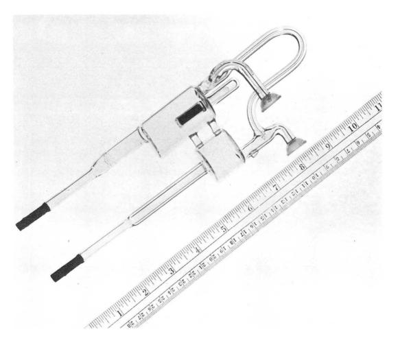
Fig. 3. Close-up photograph of mercury-plug flowmeter showing details of the capillary tip, magnetic plunger, U-shaped tube, and inlet and outlet chambers.
