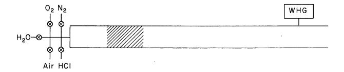
Fig. 49. Schematic drawing for the experiments to determine the effect of  $O_2$ ,  $N_2$ ,  $H_2O$ , HCl, and air on the yield of atomic hydrogen from a low-pressure discharge (Sec. V.C.2 to 5).
