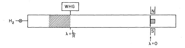
Fig. 83. Schematic drawing showing a movable probe located in a diffusion tube.
