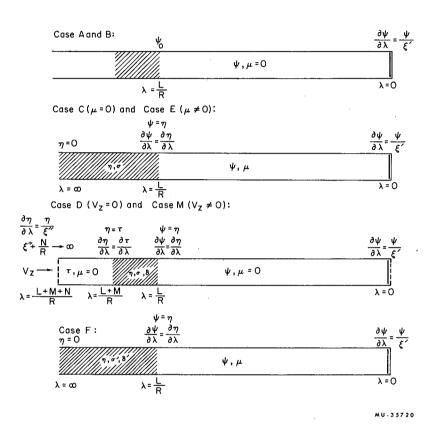
Fig. 45. Schematic drawing showing dimensionless groups and boundary conditions for Cases A to F and M.
