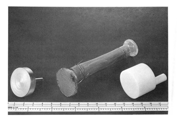
Fig. 13. Photograph of movable probes: (a) a nickel-plated copper plug (on left), (b) a Teflon plug with magnetic stirring rod (on right), and (c) a probe containing platinum mesh (not visible) and nickel-plated copper mesh to provide a large amount of catalytic surface area.
