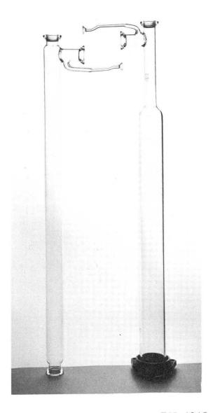
Fig. 10. Photograph of reaction tube No. 3 showing the 75-cm discharge-zone tube (on the left-hand side) and the 75-cm buffer-zone tube.
