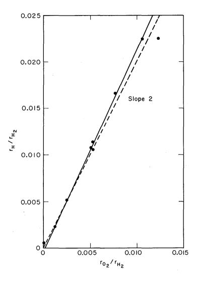
Fig. 61. The effect of low  $0_2$  flow rates on the yield of atoms from a low-pressure (80 mtorr  $\rm H_2$ ) 50-MHz discharge (20% dial setting). At least two atoms are produced per molecule of  $0_2$  added. The concentrations of H and  $0_2$  are plotted relative to the amount of  $\rm H_2$  in the entering gas stream. (January 31, 1965).
