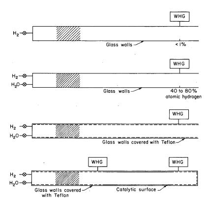
Fig. 48. Schematic drawing showing the four stages of the planned experiments: (a) verify that a discharge in pure hydrogen produces few atoms, (b) verify that the addition of water to the hydrogen increases the atom yield, (c) determine if the addition of water is a gas- or surface-phase effect, and (d) study the catalytic properties of surfaces in the presence and absence of water (if it is a surface-phase effect).
