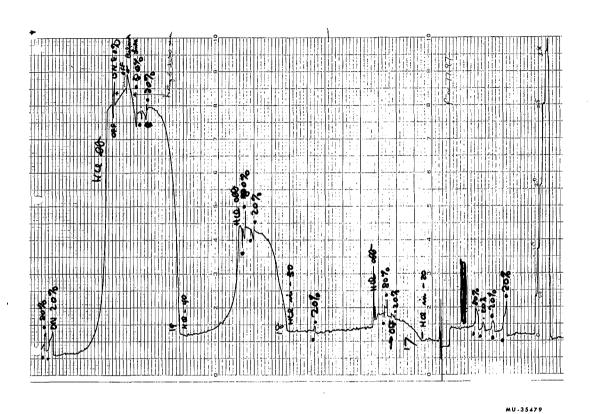
Fig. 56. Response of water-cooled WHG No. 1 (125 holes, 0.59 mtorr full scale) to the actions of adding progressively larger amounts of HCl gas and trying to produce atomic hydrogen with a 50-MHz discharge. The curves demonstrate that the HCl has no effect on the yield of atoms and that the percent dissociation in pure hydrogen is small (0.1%). P = 81 mtorr and t = 20 sec/small div (right to left). (February 2, 1965).
