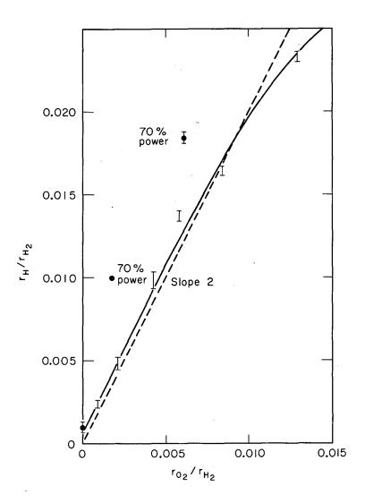
Fig. 63. The effect of low O<sub>2</sub> flow rates on the yield of atoms from a low-pressure (80 mtorr  $\rm H_2$ ) 50-MHz discharge (20% dial setting). The points corresponding to a 70% dial setting on the 50-MHz oscillator indicate that the stoichiometric ratio of two atoms per O<sub>2</sub> molecule is only a lower limit. The concentration of H and O<sub>2</sub> are plotted relative to the amount of  $\rm H_2$  in the entering gas stream. (February 7, 1965).
