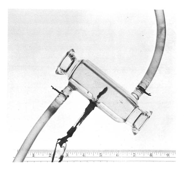
Fig. 1. Photograph of water-cooled-glass thermocouple assembly. Pyrex O-ring joints (No. 25) are used.
