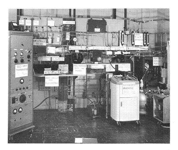
Fig. 26. Photograph of the overall flow-tube apparatus showing the 50-MHz oscillator and the 2.45-GHz diathermy machine.
