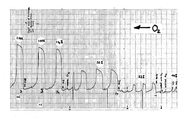
Fig. 57. Response of water-cooled WHG No. 1 (125 holes, 0.58 mtorr full scale) to 50-MHz discharge pulses (20% dial setting) with successively increasing quantities of 02 added to the hydrogen gas. The top and bottom figures show the measured atom concentration and the amount of 02 added, respectively. The yield of atoms in pure hydrogen is very low (0.06%). P=79 mtorr,  $v_z \approx 72$  cm/sec, and t = 20 sec/small div (right to left). (January 31, 1965).
