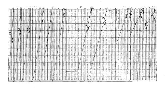
Fig. 60. Typical response of Decker micromanometer (2300 mtorr full scale) to the loss of  $O_2$  from a bulb of known volume ( $V_1 = 44 \text{ cm}^3$  and  $V_0 + V_1 = 537 \text{ cm}^3$ ). These curves show the  $O_2$  flow rate into the vacuum system and consequently the mole fraction of  $O_2$  in the hydrogen gas. Slopes Nos. 9 to 18 correspond to the discharge peaks Nos. 9 to 18 (2.8% to 16.4% atom yield) in Figs. 58 and 59. t = 20 sec/small div (right to left). (January 31, 1965).
