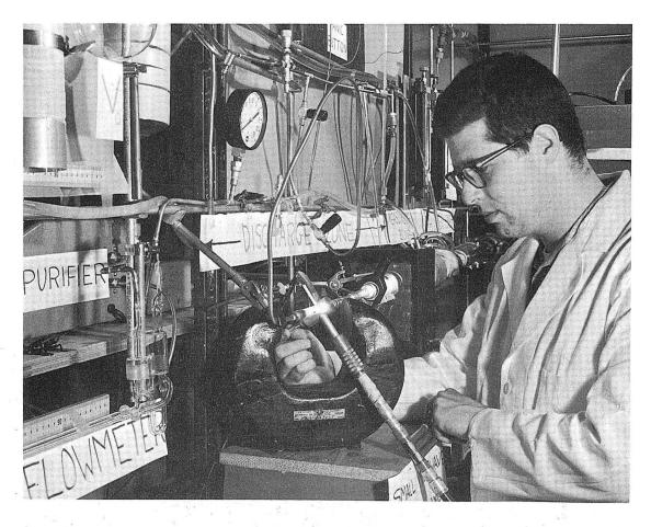
Fig. 28. Photograph showing author tuning small-diameter microwave cavity.
