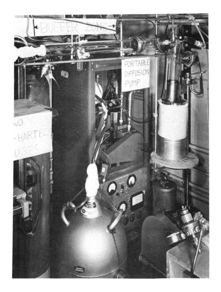
Fig. 20. Photograph of the portable diffusion pump, large-diameter liquic nitrogen trap with corrugated copper sheet (upper right corner), Kinney KC-5 mechanical pump (lower right corner), and buffer-zone tube.
