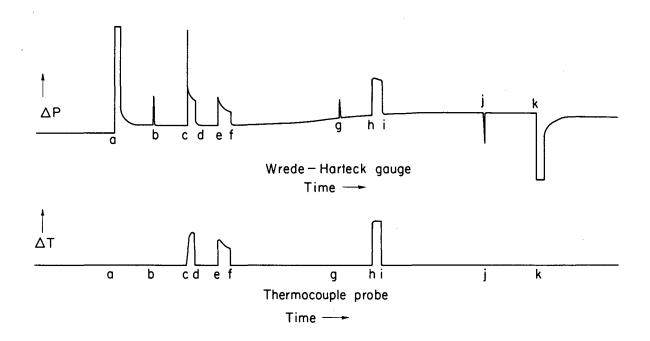
Fig. 30. Schematic diagram showing the output signals of a Wrede-Harteck gauge and a thermocouple probe resulting from various perturbations in the flow system.
