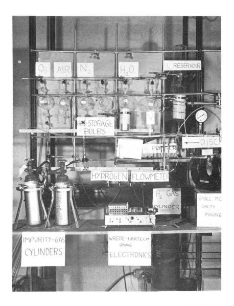
Fig. 5. Photograph of the gas-handling system, including the gasstorage bulbs, the known-volume bulb ( $\rm V_{o}$ ), and the hydrogen purifier, reservoir, and flowmeter.
