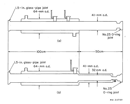
Fig. 7. Schematic drawings of (a) reaction tube No. 1, and (b) reaction tube No. 2.
