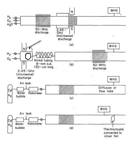
Fig. 67. Schematic drawing showing four critical experiments to determine the effect of water on the yield of atomic hydrogen from a low-pressure discharge: (a) the effect of different discharges; (b) the effect of the upstream conversion of oxygen to water; (c) the effects of cylinder hydrogen, a water bubbler, and an air leak in the rotameter; and (d) the response of different measurement devices to the effect of water.
