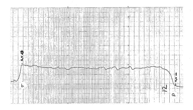
Fig. 51. Response of water-cooled WHG No. 1 (125 holes, 0.7 mtorr full scale) to the actions of (a) adding a small amount of water to the hydrogen gas, and (b) stopping the addition of water. The effect persisted for 50 minutes and showed no tendency to decay. This curve strongly suggests that the presence of water alters the effusion equilibrium within the WHG, although other explanations are also possible. P = about 75 mtorr and t = 20 sec/small div (right to left). (February 2, 1965).
