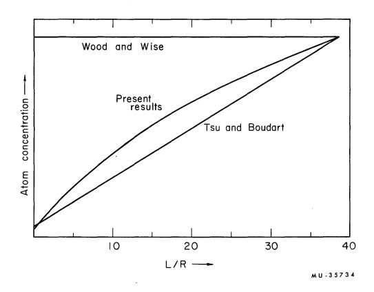
Fig. 84. Schematic drawing illustrating the concept of experiments performed to demonstrate the effect of a catalytic probe on the atom concentration at the discharge boundary. According to present theories on the subject, movement of a highly catalytic probe would have either no effect (Wood and Wise), a linear effect (Tsu and Boudart), or a non-linear effect (present results).
