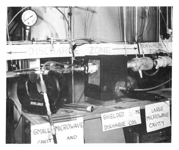
Fig. 19. Photograph of the reaction-tube No. 3 discharge zone and the small-diameter microwave cavity and magnetron magnet (on left), the shielded 50-MHz output LC circuit (center), and the largediameter microwave cavity (right).
