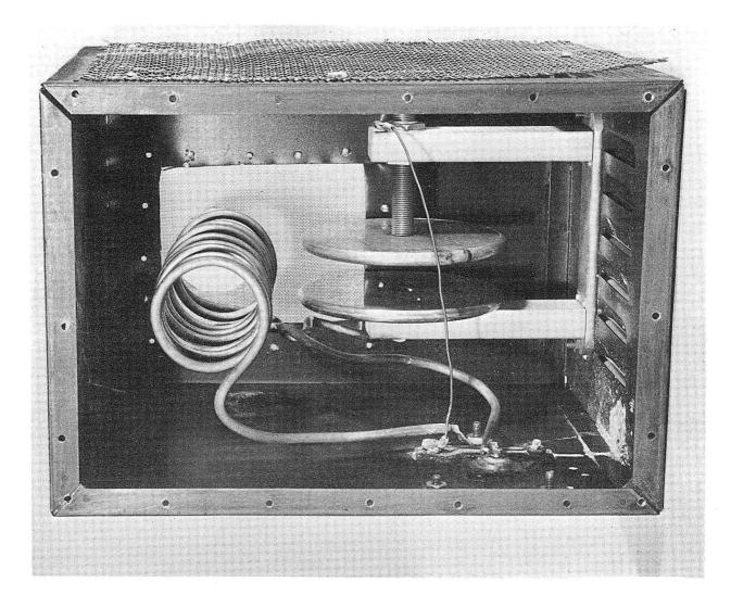
Fig. 17. Photograph of output LC circuit and shielded enclosure.
