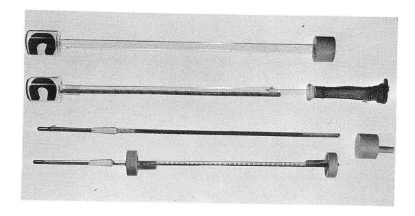
Fig. 2. Photograph of movable probes. From top to bottom they are (a) a magnetically moved glass-tube and Teflon-sleeve assembly to hold metal or glass disks, (b) a magnetically moved glass-tube assembly to hold a probe containing platinum mesh and nickel-plated copper mesh, (c) a 360°C thermometer with an electroplated nickel end, (d) a magnetically moved 360°C thermometer with an AgNO<sub>3</sub>-coated, and (e) a magnetically moved Teflon plug (on lower right-hand side).
