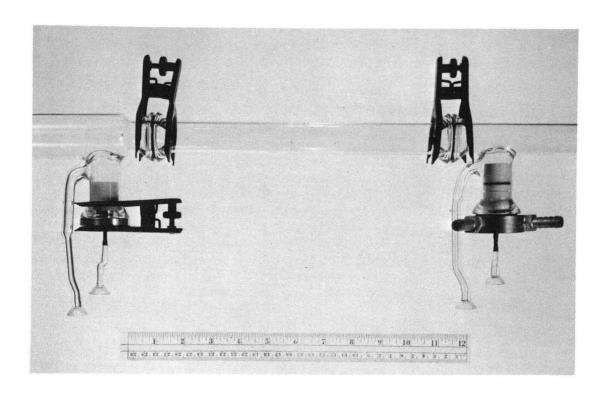
Fig. 29. Close-up photograph of the central portion of reaction tube No. 3 showing the (a) non-water-cooled WHG fitting (located in the left WHG port), (b) water-cooled WHG fitting (located in the right WHG port), and (c) an intermediate glass section constructed to determine the recombination coefficient of atomic hydrogen on metals (vapor plated on the inside of the glass tube).
