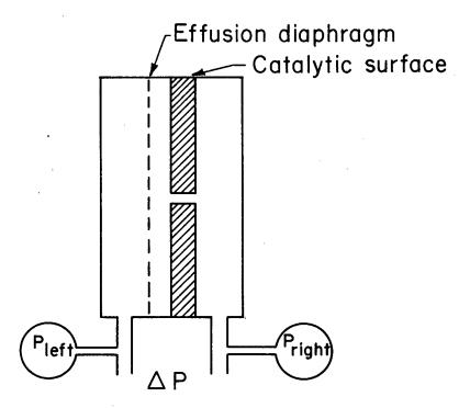
Fig. 31. Schematic drawing of a Wrede-Harteck gauge atom-concentration-to-pressure transducer. The catalytic surface is on the right-hand side of the effusion diaphragm.
