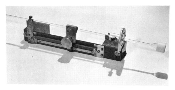
Fig. 15. Photograph of Wilson-seal and ratchet assembly.
