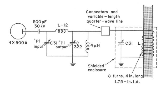
Fig. 16. Schematic diagram of pi network of 50-MHz oscillator and output LC circuit; L has eight turns of 1/4-in. o.d. copper tubing, is 4 in. long, and has an i.d. of 1.75 in.
