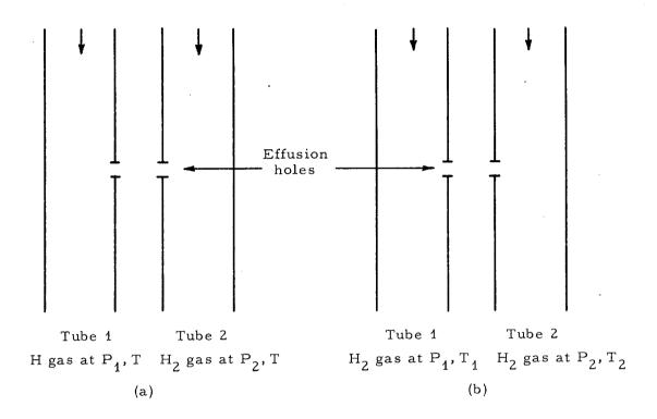
Fig. 33. Schematic drawing flow tubes (each with an effusion hole) used to demonstrate the principles of a Wrede-Harteck gauge: (a) isothermal system, and (b) non-isothermal system.
