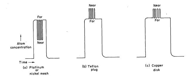
Fig. 93. Schematic drawing showing the results of experiments with the (a) platinum-mesh and nickel-plated copper-mesh probe, (b) Teflon plug, and (c) copper disk. The words near and far refer to the distance between the probes and the discharge boundary.
