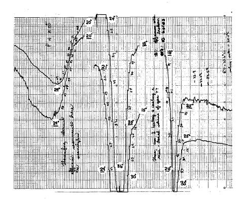
Fig. 37. Response of water-cooled WHG No. 1 (split diaphragm, 0.54 mtorr full scale) and WHG No. 2 (10 holes, 0.50 mtorr full scale) to identical changes (assumed) in the water temperature. These curves demonstrate the disturbing influence of thermal effusion on a WHG. P = 56 mtorr and t = 20 sec/small div (right to left). (March 30, 1965).
