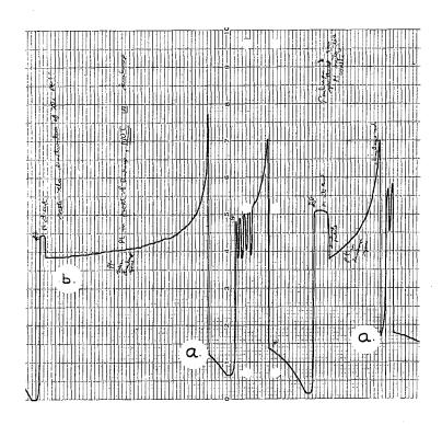
Fig. 86. Curves similar to those shown in Fig. 85, demonstrating the effect of a movable Pt probe on the atom concentration near a microwave discharge, and also the effect of the presence of small amounts of air on the yield of atomic hydrogen from the discharge. The discharge was turned on continuously until at point (b) it was turned off. This action poisoned the Pt probe, as is shown by the smaller height of the spikes in Fig. 87. t = 20 sec/small div (right to left). (November 29, 1964).
