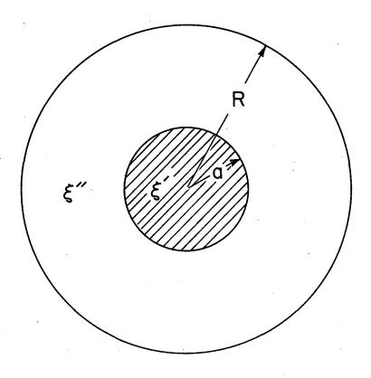
Fig. 47. Schematic drawing of the composite catalytic end plate. The inner disk is the more reactive of the two materials.
