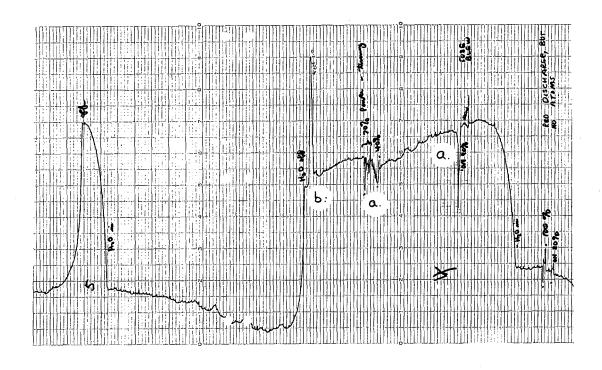
Fig. 54. Response of water-cooled WHG No. 1 (125 holes, about 0.5 mtorr full scale) to the actions of (a) operating the 50-MHz oscillator at 40%, 70%, and 90% dial settings after adding > 0.16% water to the hydrogen gas, and (b) electrostatically applying a 0.25 mtorr "pressure" pulse. The curve shows that water has no effect on the yield of atoms from the discharge. P = 78 mtorr and t = 20 sec/small div (right to left). (February 1, 1965).
