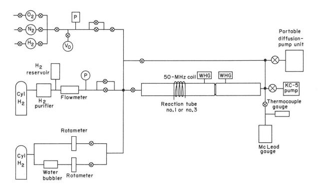
Fig. 25. Schematic drawing of flow-tube apparatus. Either the small-diameter or large-diameter microwave cavities could be operated independently of the 50-MHz discharge. Both rotameters leaked.
