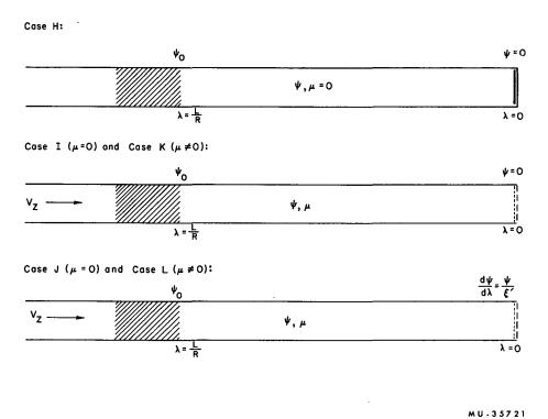
Fig. 46. Schematic drawing showing dimensionless groups and boundary conditions for Cases H to L.
