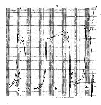
Fig. 39. Response of water-cooled WHG No. 1 (split diaphragm, 0.50 mtorr full scale) and WHG No. 2 (10 holes, 0.62 mtorr full scale) to identical changes (assumed) in atom concentration. The ratio of the gauge responses is (a) 1.30, (b) 1.20, and (c) 1.20, which indicates that a WHG may not be an absolute device even at low pressures. P = 37 mtorr and t = 20 sec/small div (right to left). (April 2, 1965).
