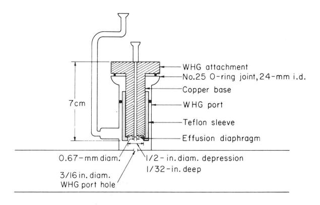
Fig. 34. Schematic drawing of the WHG fitting, the WHG port, and the WHG port hole.
