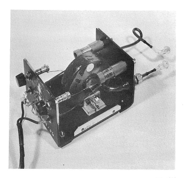
Fig. 23. Close-up photograph of modified Decker 306-2A pressure sensor. The ionization transducer has been replaced by a tuned capacitance bridge. The residual volume of the connecting stainless-steel tubing and glass ball joints can be considerably decreased.
