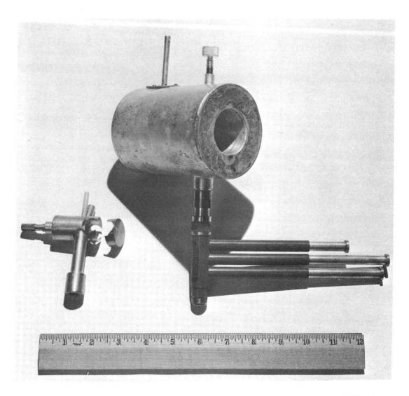
Fig. 18. Photograph of small-diameter and large-diameter microwave cavities and triple-stub tuner.
