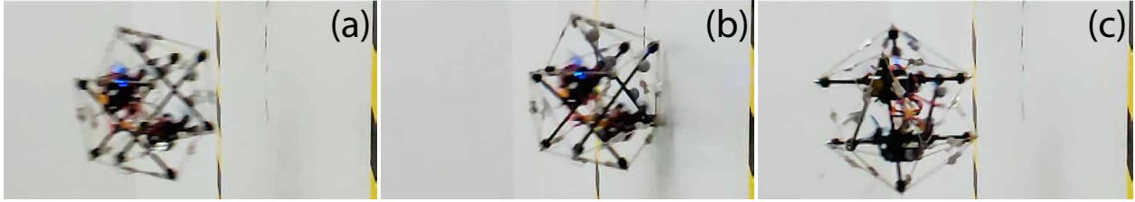
Figure 3.10: Sequence of images showing the process of a collision against a concrete wall: (a) Vehicle accelerates towards the wall. (b) Vehicle comes to a full stop. (c) Vehicle bounces back from the wall. The collision speed is 7.8m/s.
