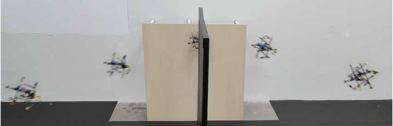
Figure 4.7: Composite image of the tracking experiment. The quadcopter tracks a trajectory from left to right while avoiding the black obstacle in the middle of the space. For the collision-inclusive trajectory, the quadcopter takes advantage of a collision with the yellow obstacle in the back. The distance between the shown left-most state and right-most state is about 2m.
