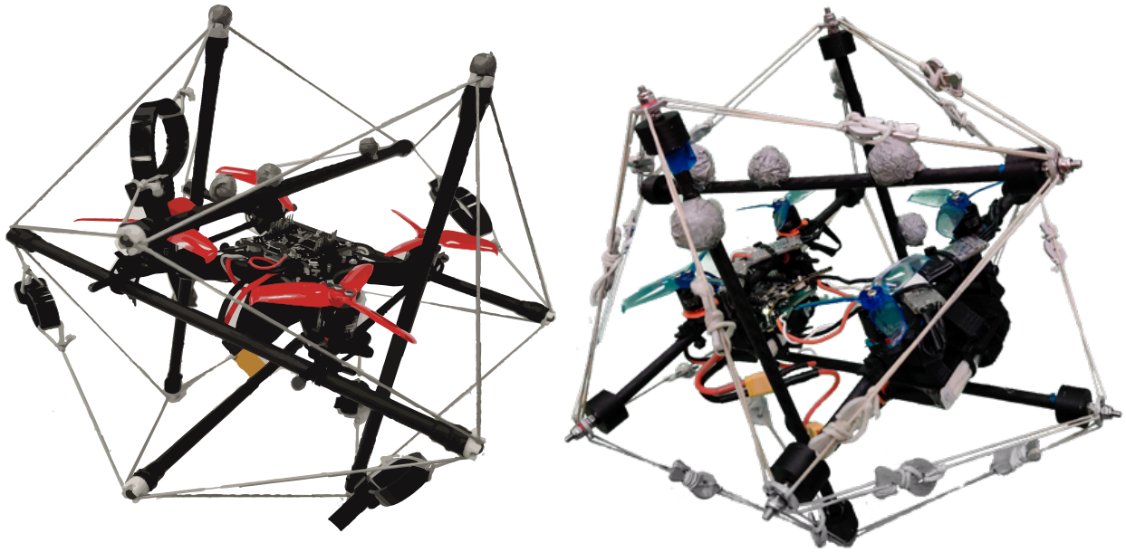
Figure 3.1: The icosahedron tensegrity aerial vehicles. Left: stage one experimental vehicle, built with a miniature quadcopter attached to a tensegrity shell. Right: stage two experimental vehicle, all electronics of which are directly mounted on the tensegrity rods. Both vehicles are built with carbon fiber rod of 20cm length.
