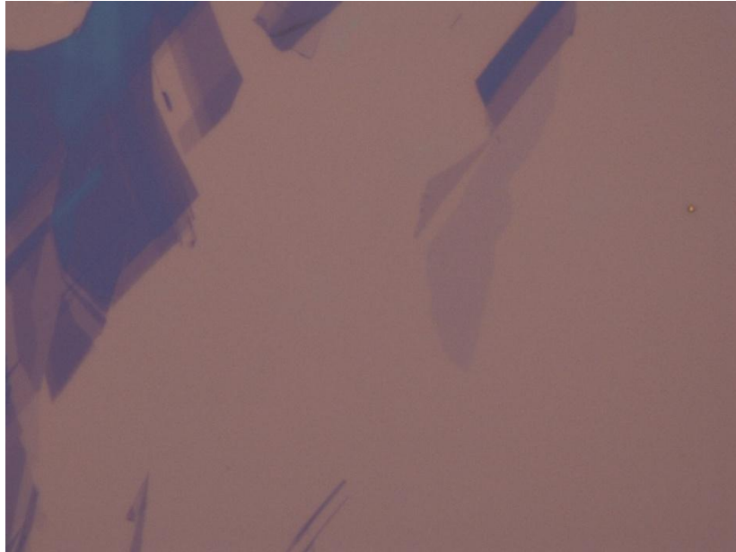
Figure 2.3 Optical microscope image of graphene sample prepared by mechanical exfoliation method in the Nano-Device Laboratory, UCR.
