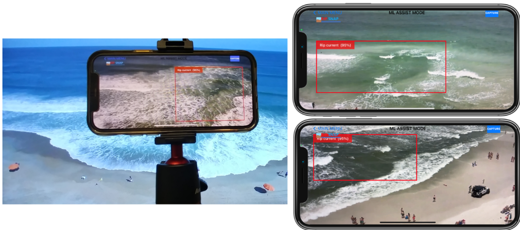
Figure 4.5: Appearance of the RipSnap app with examples of rip currents detected by the app. The location of the rip current is visualized using the red bounding box with the label and the confidence score of detection.
