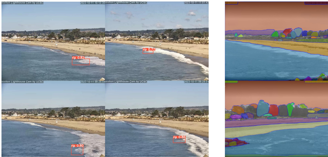
Figure 8.3: Automated rip current data collection and shoreline segmentation from wireless network camera.
