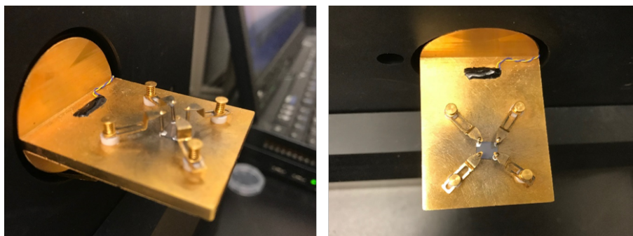
Figure 2.13: Hall-effect measurement setup. (a) Side view (b) top view
