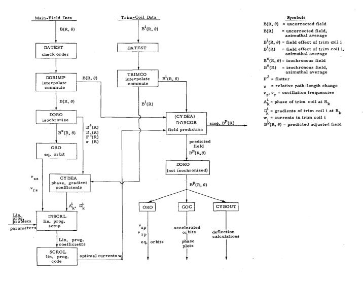
Fig. 1. Schematic diagram of trim-coil adjustment computation.
