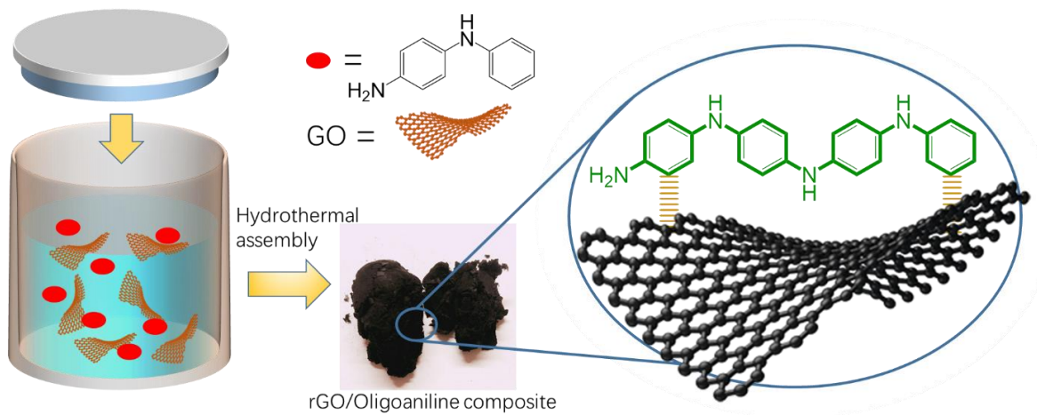
Scheme 4.1 Illustration of the hydrothermal synthesis of rGO-OANI composites.
