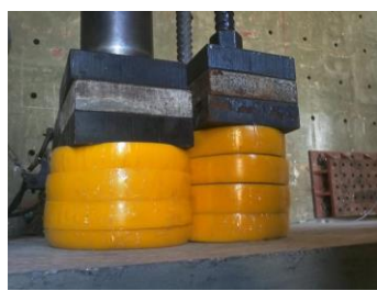
Figure 3.10 – Polyurethane bearing of Unit 1B: (a) components; (b) single pad; (c) assembled bearings.
