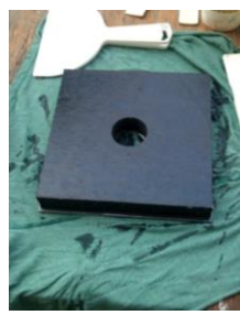
Figure 3.9 – Rubber bearing of Unit 1A: (a) components; (b) single pad; (c) assembled bearings.
