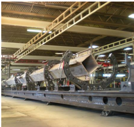
ConXTech fabrication shop with rotating clamps www.prweb.com/releases/conxtech/ladbs-approved/prweb10762433.htm
