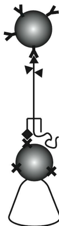
Figure 3-2. Optical tweezer manipulation of the twPNA-DNA-dig complex, which is attached by one end to an anti-digoxigenin-coated sphere, manipulated by the optical trap, and by the other end to a streptavidin-coated sphere, sucked onto a micropipette.
