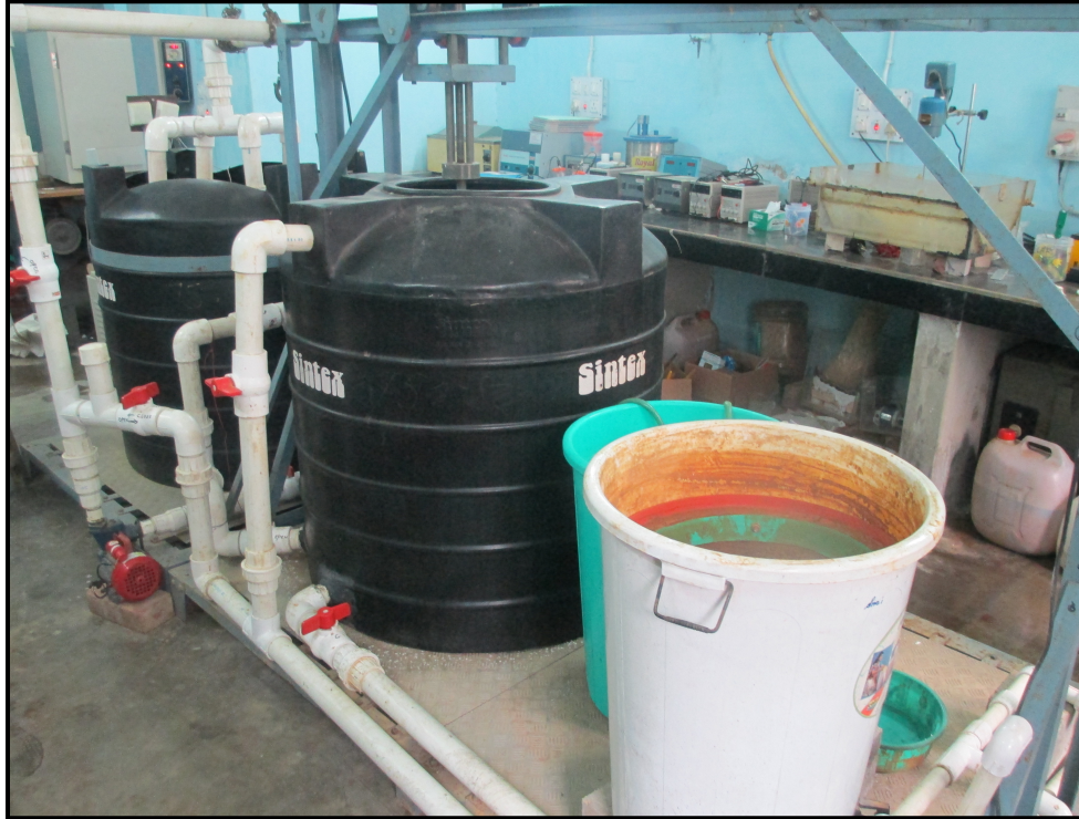
Figure 1.3: 700 L electrocoagulation field prototype in Kolkata, India (Photo: C. van Genuchten)
