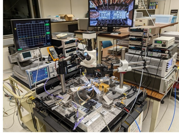
Figure 4.14: Transmitter continuous wave (CW) testing setup.
