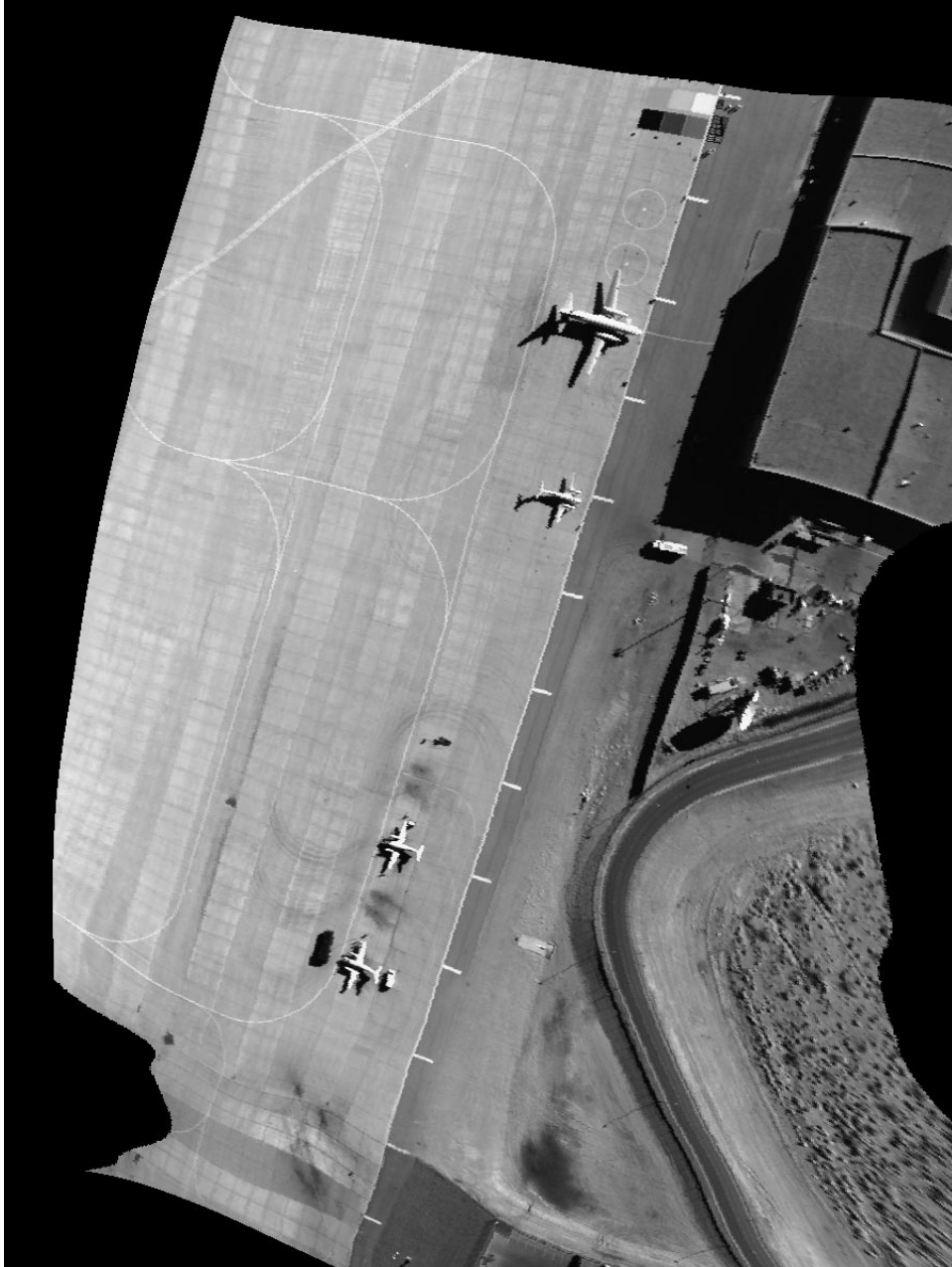
Third Order Polynomial and Reciprocal Multiquadric Two-Stage Image Registration. Origin (1,1) at the center of the pixel in the upper left corner of the reference coordinate system. Image extents shown here are: upper left (601,1) and lower right (2400,2400).
