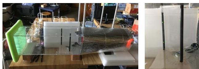
Fig 9. Experimental setup for our sensing systems in a duct
