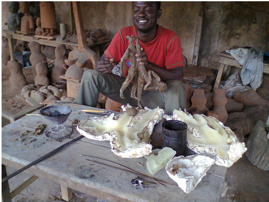
Fig. 2. Plaster of Paris Negative Mould with Silicon Used as Positive Mould.
