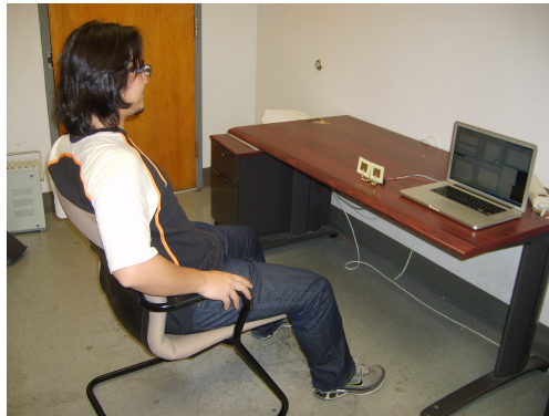
Figure 3.8: The Doppler radar measures vital signs from a subject.
